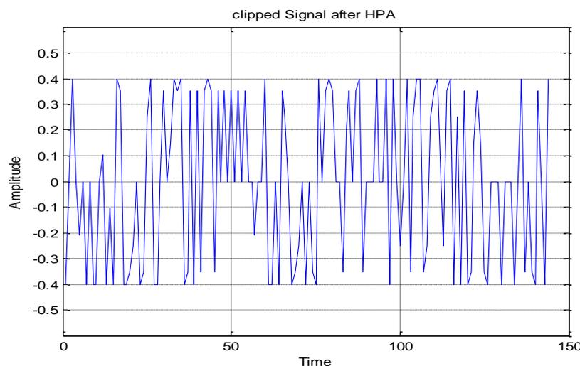
**Figure 5** OFDM signal with clipping at N=1024
