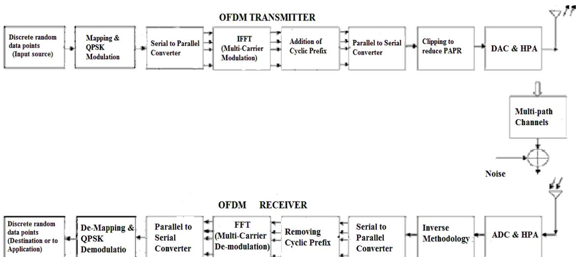
Figure 1 OFDM signal transmission and reception block diagram
