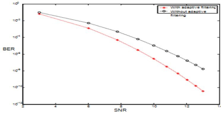
**Figure 12** SNR vs BER for SNR = 20 and Samples=10
