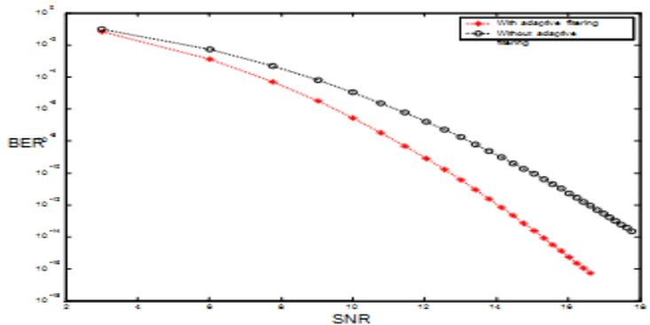
**Figure 14** SNR vs BER for SNR = 30 and Samples=10
