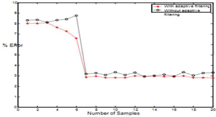
**Figure 11** No. of Samples vs Error when SNR = 30 and Samples=20
