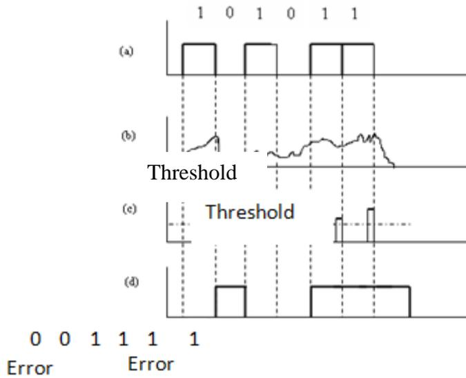
**Figure 2** (a) Ideal receiver current (b) Actual current (c) Sampled current (d) resulting data pattern
