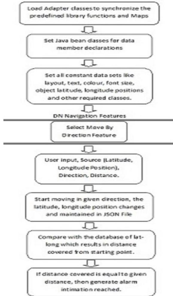
**Figure 6** Flow chart of Move by Direction
