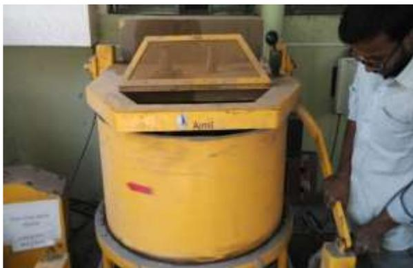
**Figure 1** Mixing Process with Pan Mixer
