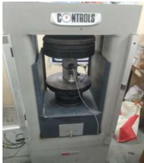
**Figure 4** Compression Testing Machine Setup
