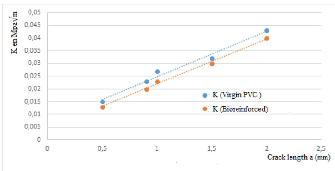
**Figure 8** Evolution of digital "K" as a function of the fault length
