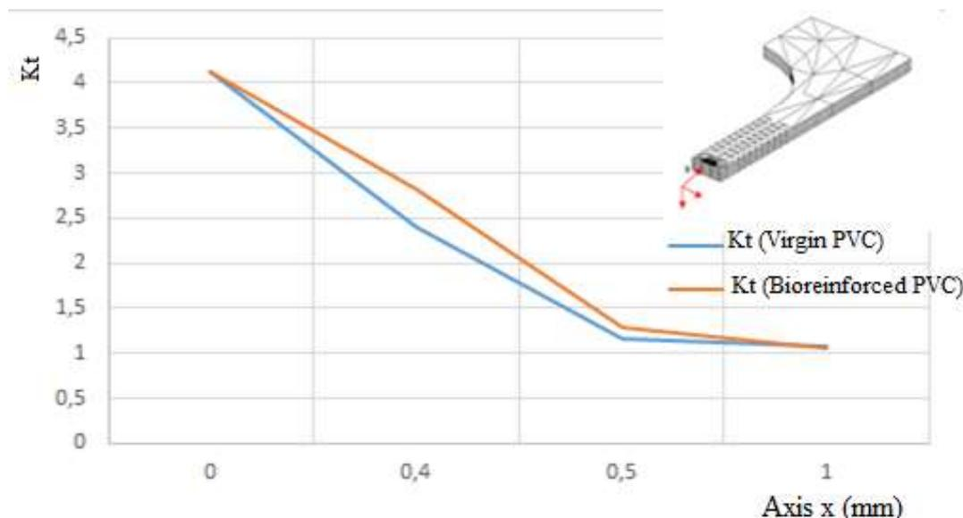
**Figure 7** Evolution of the numerical stress concentration coefficient on the horizontal axis
