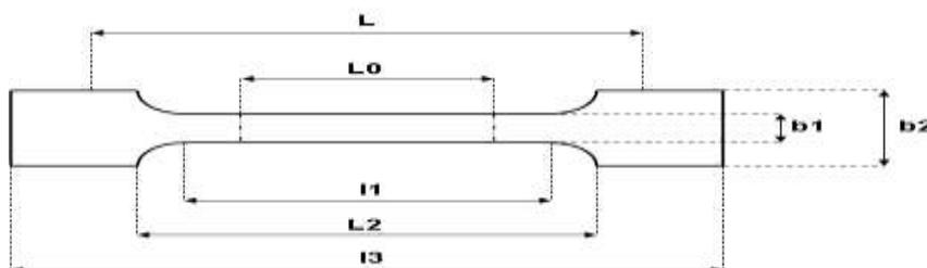
Figure 1 Specimen geometry
