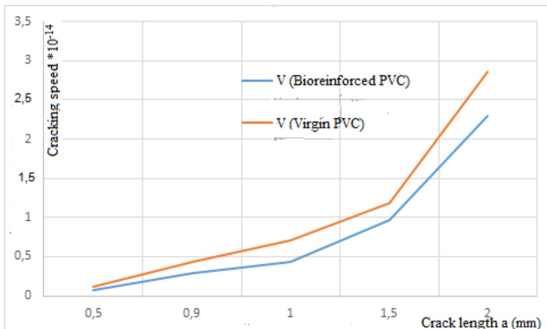
**Figure 9** Evolution of K according to the progress of the crack
