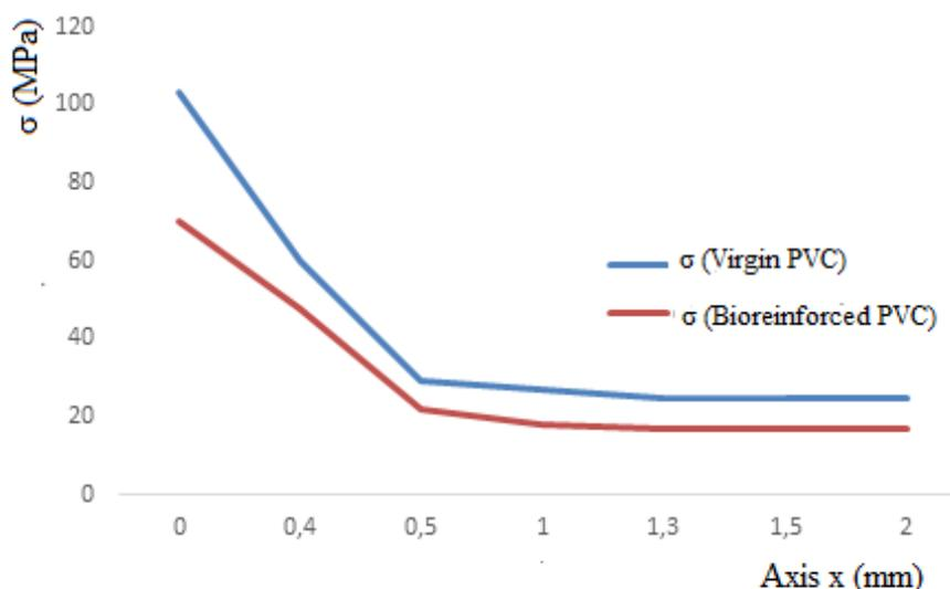
**Figure 6** Evolution of the numerical stress along the horizontal axis of the specimen
