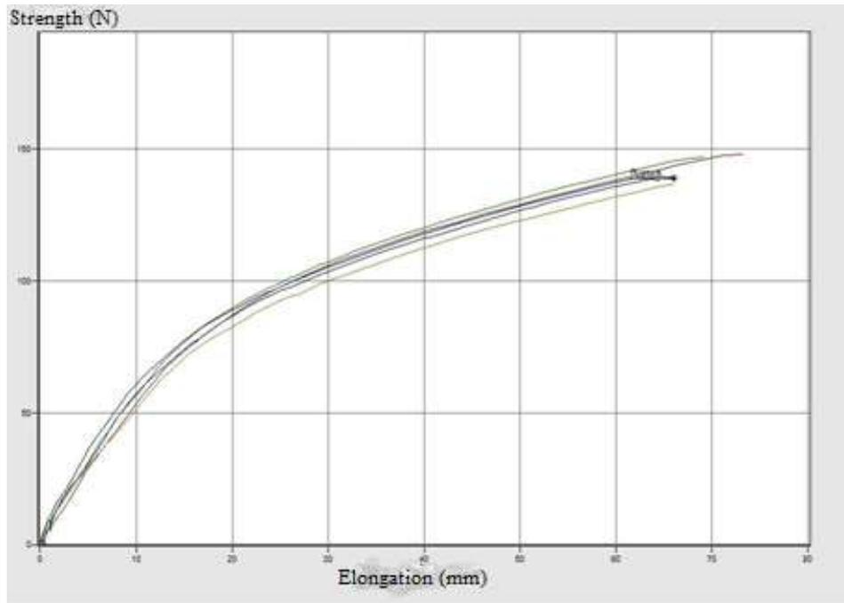
**Figure 2** Traction curves of soft PVC
