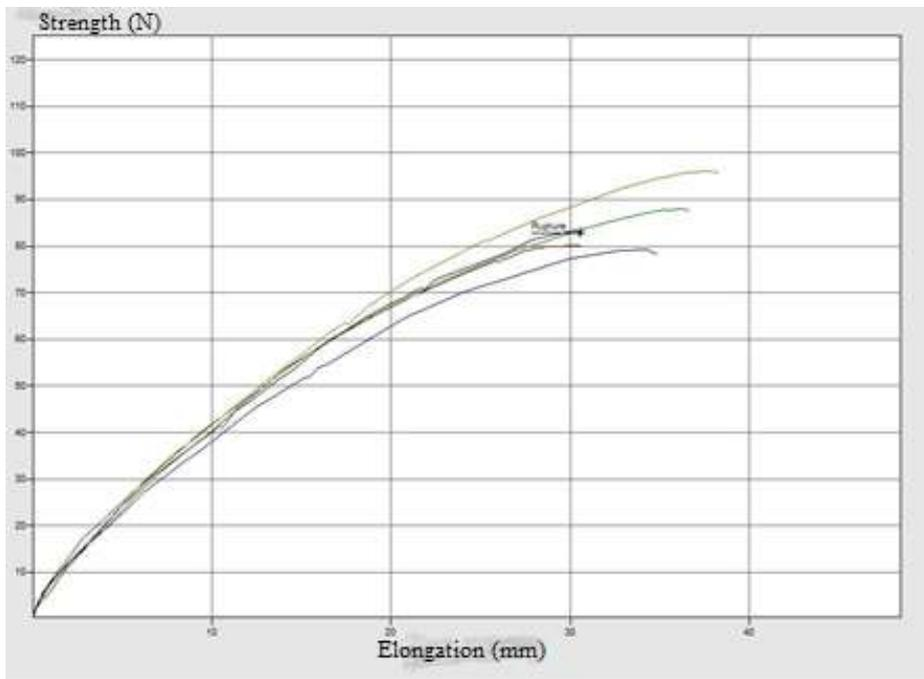
**Figure 3** Traction curves of bio-loaded soft PVC
