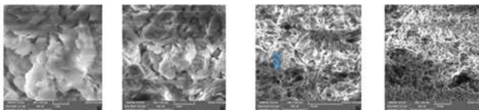
Figure 4 Scanning Electron Microscope- Energy Dispersive Spectroscopy (SEM-EDX) tipe TESCAN 3VEGAActivation ofNatural Zeolite (100 °C, 200 °C, 300 °C dan 400 °C)
