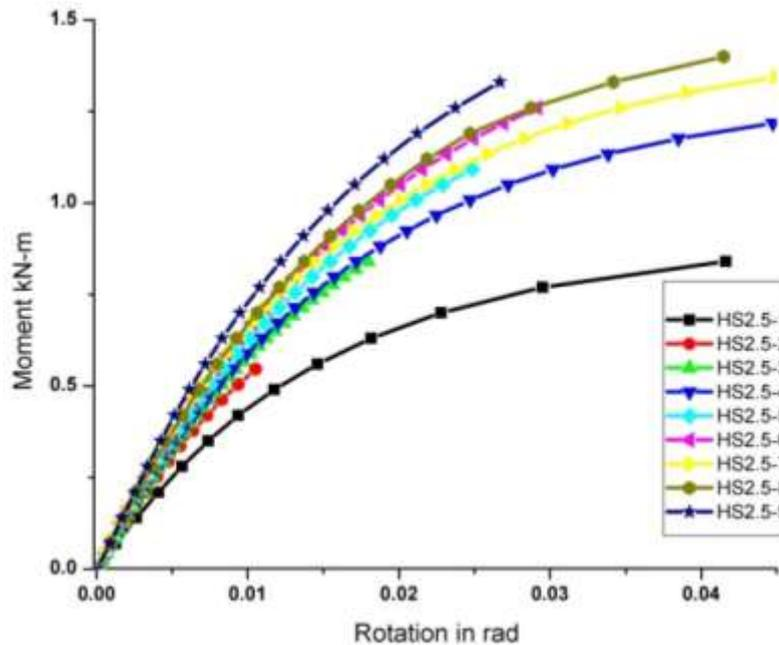
**Figure 11** Moment – rotation behavior of joint
