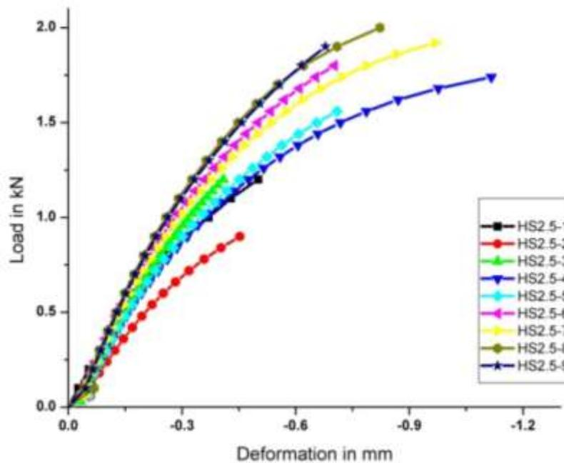
Figure 8 Bolt deformation in Compression
