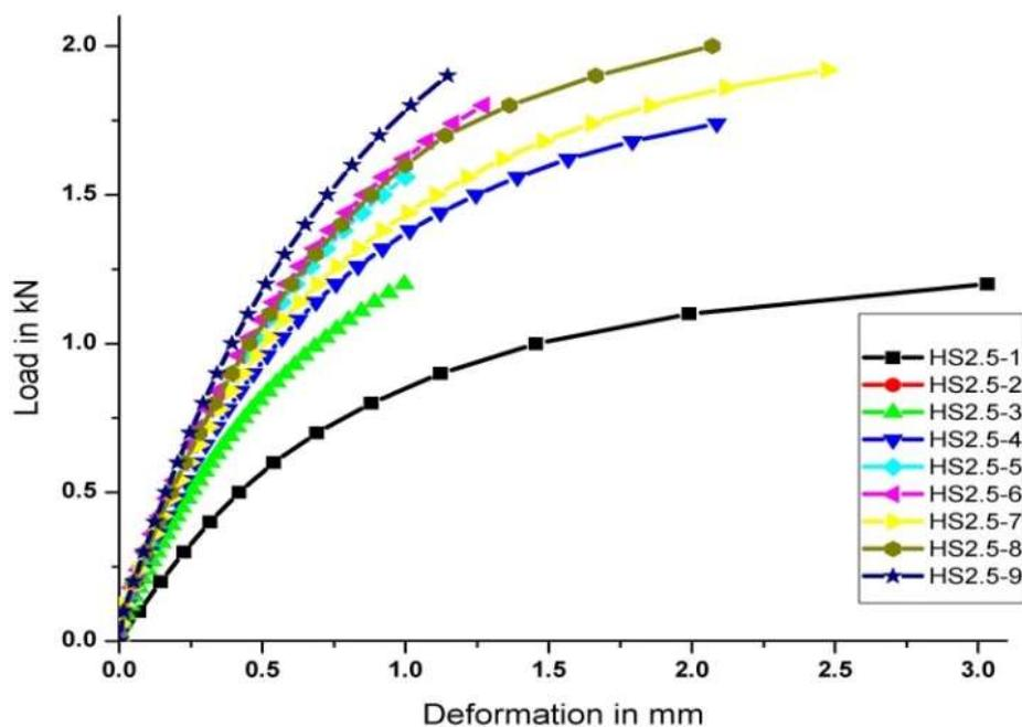
**Figure 4** End Plate deformation in Tension
