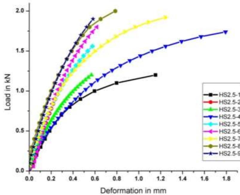
Figure 7 Bolt deformation in Tension
