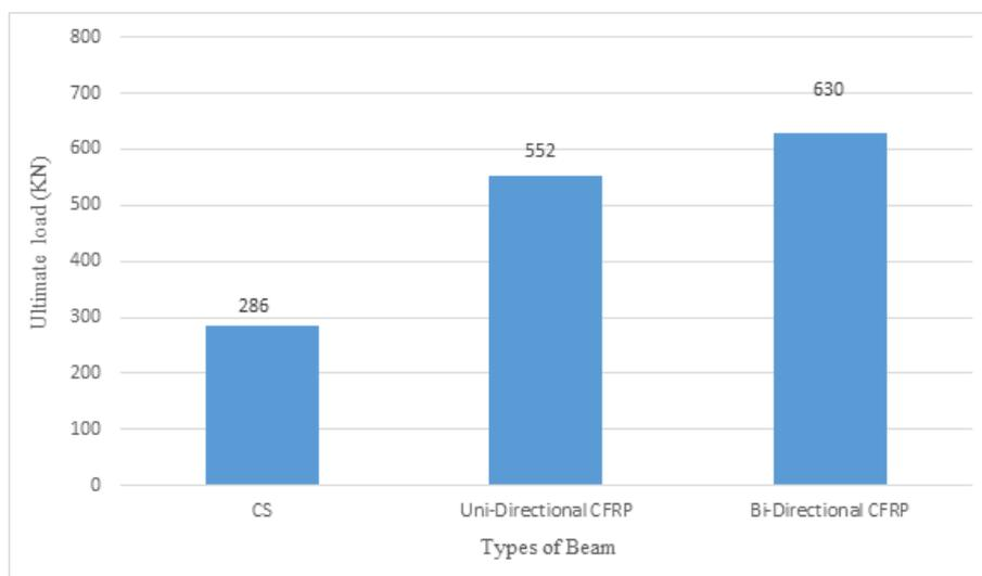
**Figure 9** Comparison of Ultimate Load Capacity
