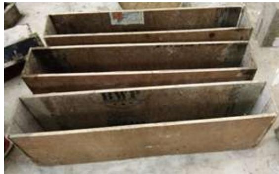
Figure 3 Plywood mould
