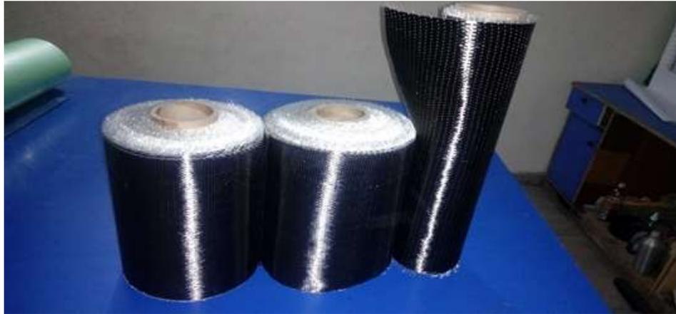
**Figure 1** Uni-directional and bi-directional Carbon fibre sheets.
