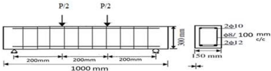
Figure 4 Geometry, Detail of reinforcement and loads of the beams.
