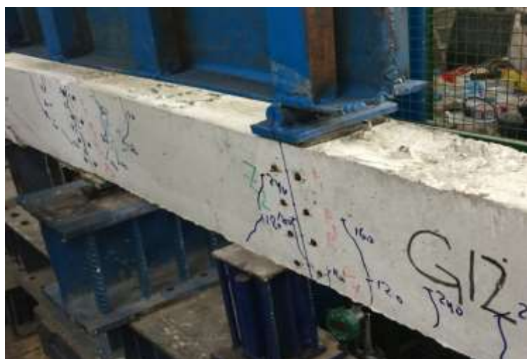
Figure 10 The patterns crack of beam G12.
