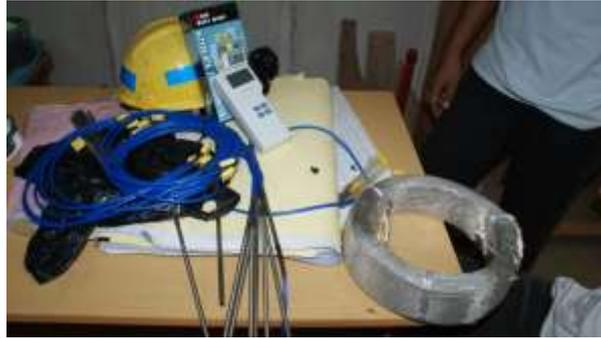
**Figure 7** Thermocouple and Digital thermometer
