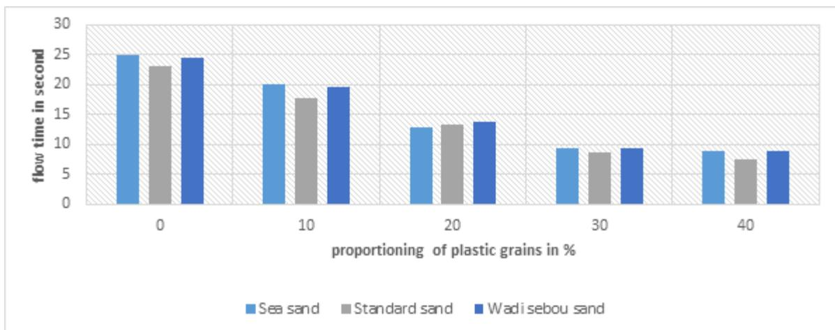
**Figure 6** The effect of adding plastic grains on the fluidity of fresh concrete
