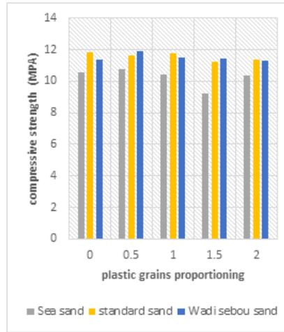
**Figure 9** the evolution of concrete compressive strength using plastic grains in 2 days
