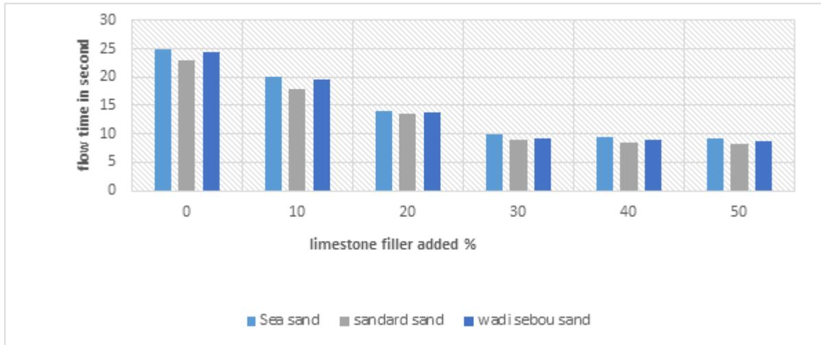
**Figure 4** The effect of adding limestone filler on the fluidity of fresh concrete
