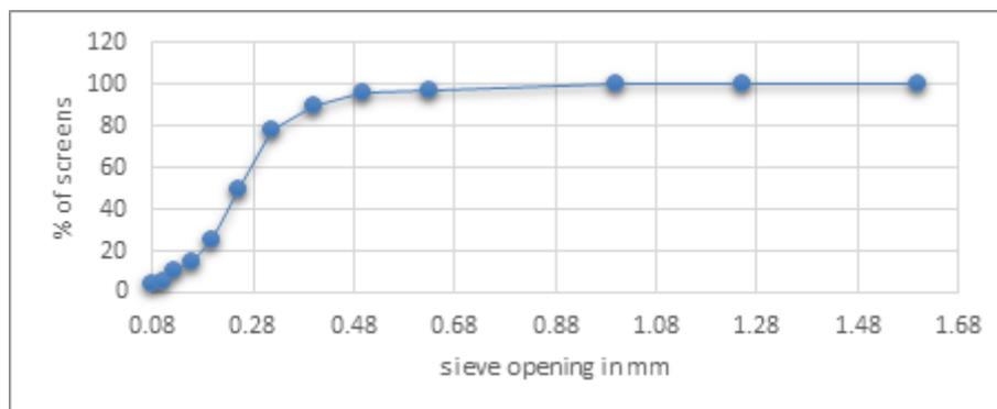
**Figure 1** The grain size curve of the river of Sebou sand
