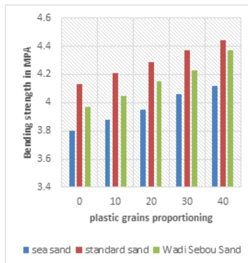
**Figure 13** the evolution of concrete bending strength using plastic grains in 2 days
