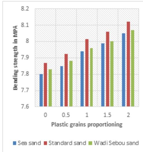
**Figure 14** the evolution of concrete bending strength using plastic grains in 28 days
