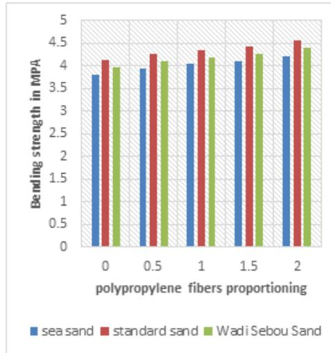
**Figure 11** the evolution of concrete bending strength using polypropylene fibers in 2 days
