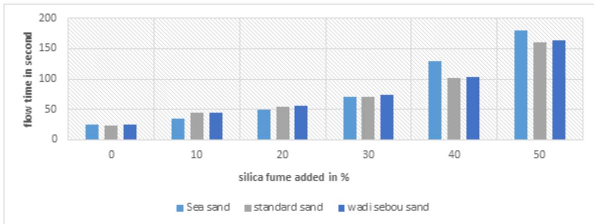
**Figure 5** The effect of adding silica fume on the fluidity of fresh concrete
