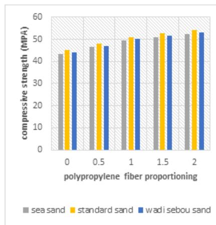
**Figure 8** The evolution of concrete compressive strength using polypropylene fibers in 28 days
