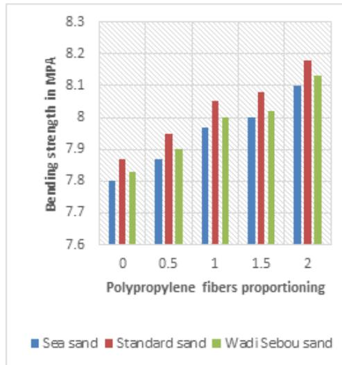
**Figure 12** the evolution of concrete bending strength using polypropylene fibers in 28 days
