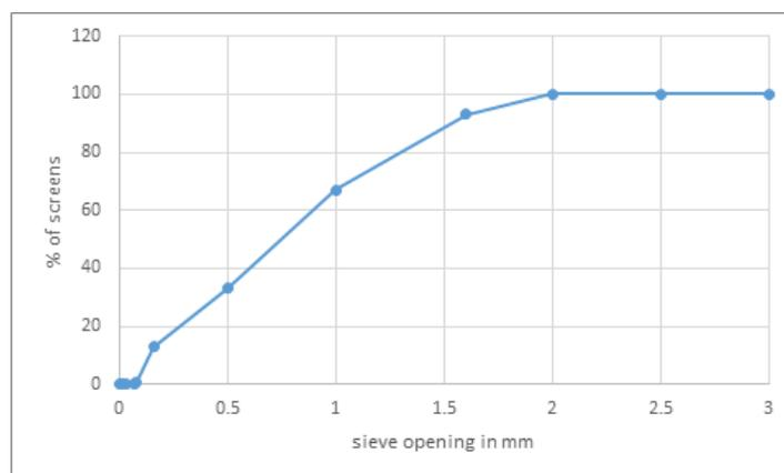
**Figure 3** The grain size curve of the standard sand
