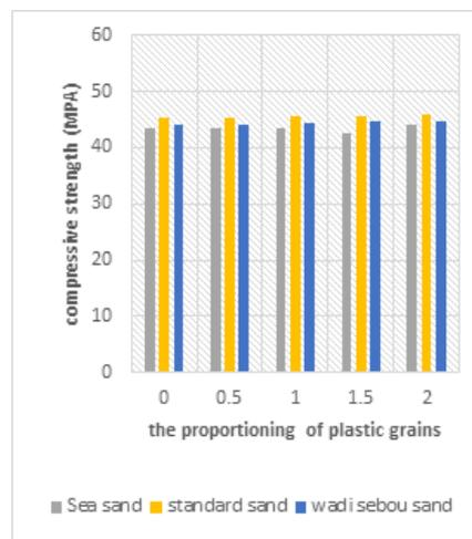
**Figure 10** the evolution of concrete compressive strength using plastic grains in 28 days
