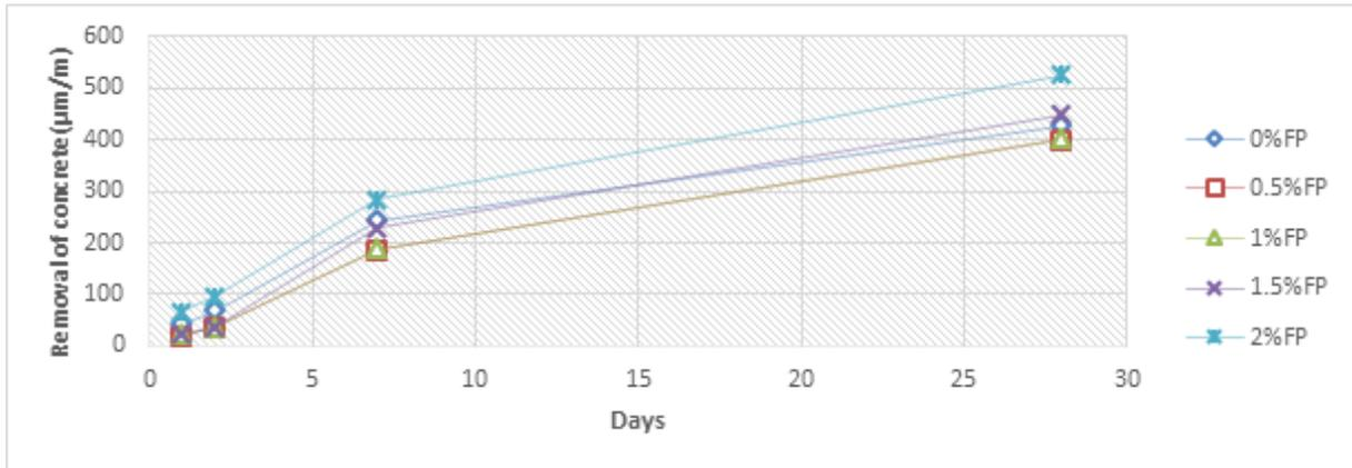
**Figure 19** Removal of the standard sand concrete with polypropylene fiber
