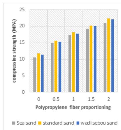
**Figure 7** The evolution of concrete compressive strength using polypropylene fibers in 2 days
