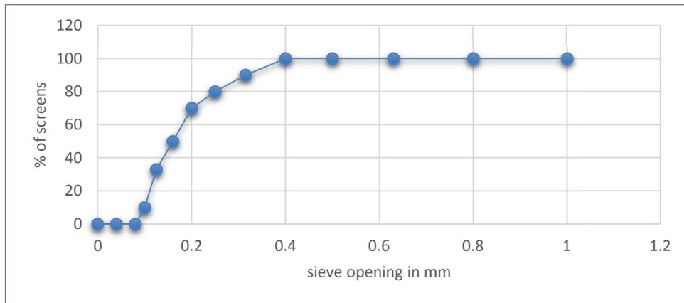
**Figure 2** The grain size curve of the sea sand
