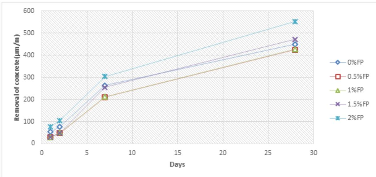
**Figure 20** Removal of the sea sand concrete with polypropylene fiber
