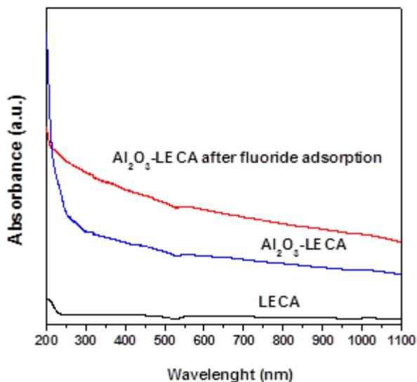
Figure 3 UV Spectra showing fluoride adsorbed on LECA
