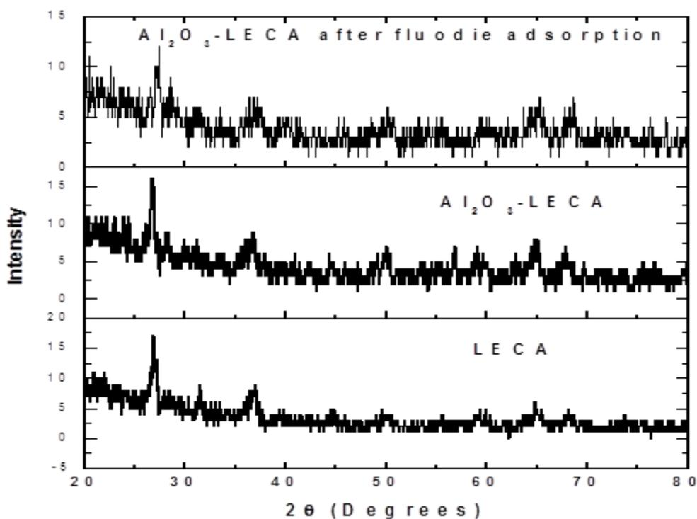
Figure 4 XRD peaks showing fluoride adsorbed on LECA
