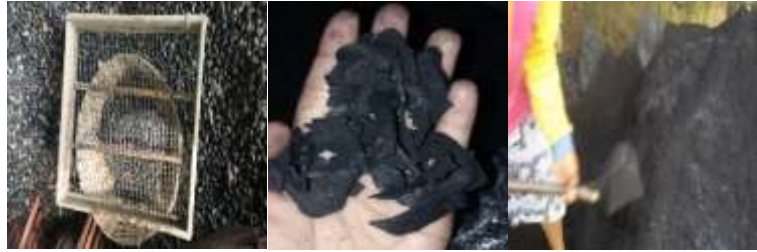
Figure 1 Filter materials (Gravel 12,5 mm, Charcoal 2 mm and Sand 2 mm)
