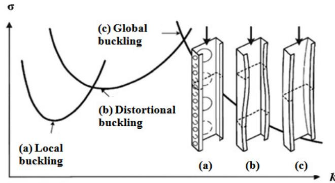
**Figure 2** Single column buckling stress  $\sigma$  versus half-wave length  $k$  and buckling form under vertical load: (a) local buckling, (b) distortional buckling and (c) global buckling [15]
