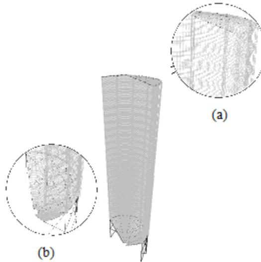
**Figure 8** Established finite element model (a) zoom on Roof-Stiffener zone and (b) zoom on Hooper-Support zone
