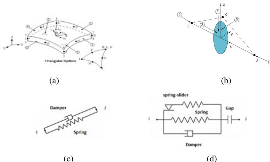
**Figure 5** Finite elements used (a) for the silo wall, (b) for the support, (c) and (d) for the lead-plug bearing [15]
