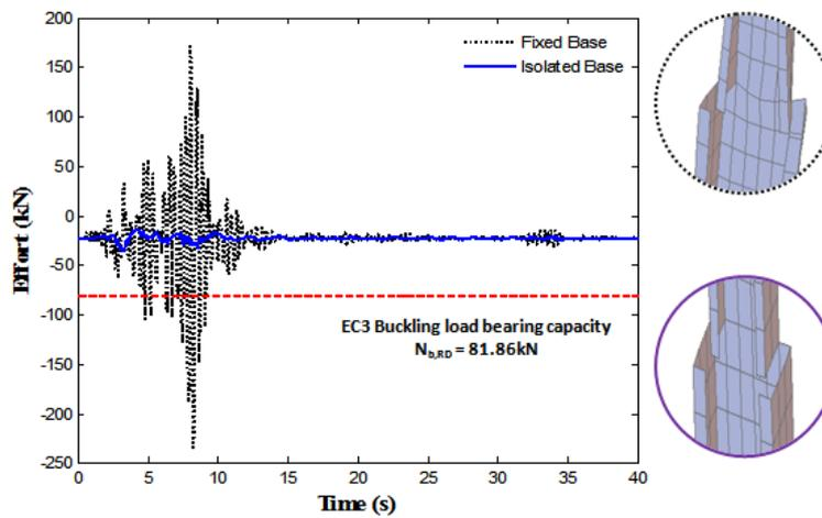
**Figure 12** Stability of top stiffener under the 1970 San Fernando ground motion
