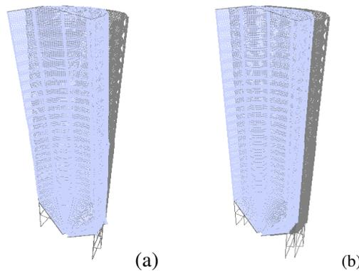
**Figure 9** Modal deformed shape (a) Fixed-base and (b) Isolated-base
