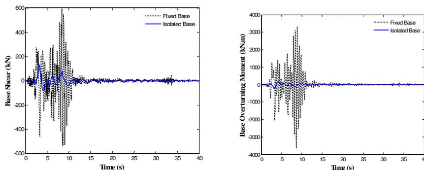
**Figure 10** Time variation of (a) base shear force and (b) overturning moment under the 1970 San Fernando ground motion for the fixed-base and the isolated silo
