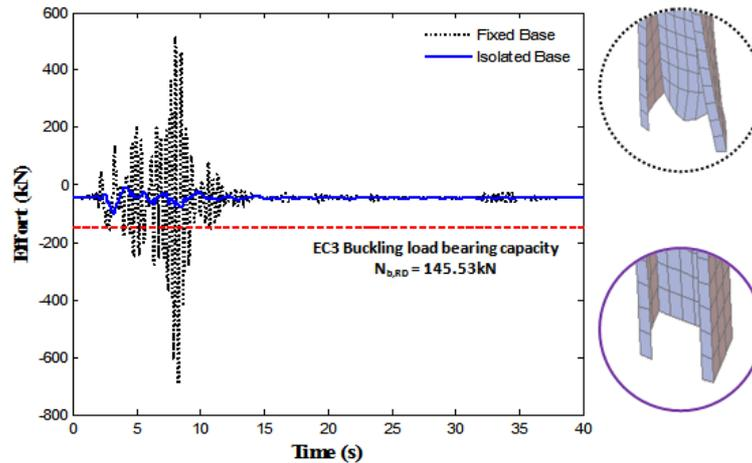
**Figure 13** Stability of bottom stiffener under the 1970 San Fernando ground motion
