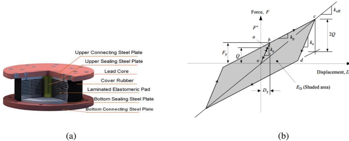
**Figure 6** Lead-plug bearings (a) Components and (b) Bilinear model [20], [21]
