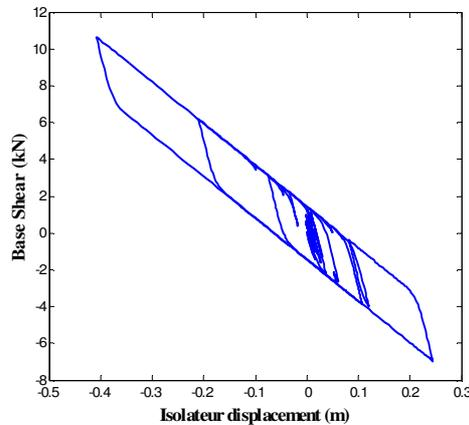
**Figure 11** Hysteresis curve of lead rubber bearing under the 1970 San Fernando ground motion
