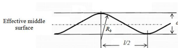
**Figure 3** Corrugation profile and geometric parameters [16]
