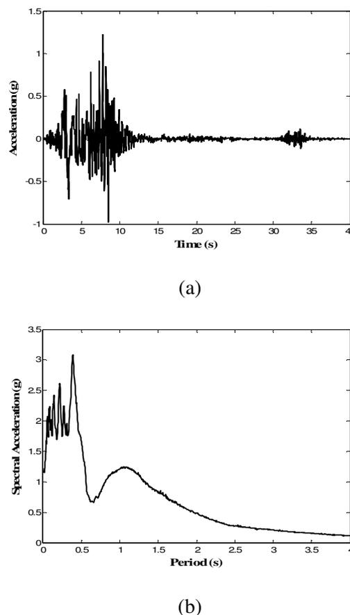
**Figure 7** San Fernando 1970 earthquake (a) ground acceleration time histories and (b) spectral acceleration
