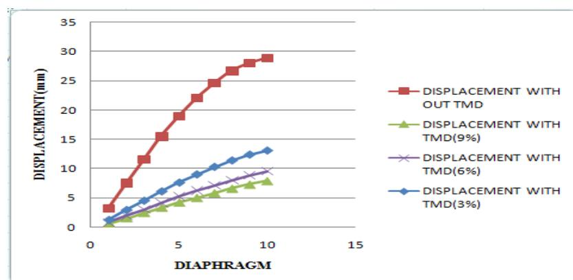
**Graph 1** Diaphragm versus Displacement
