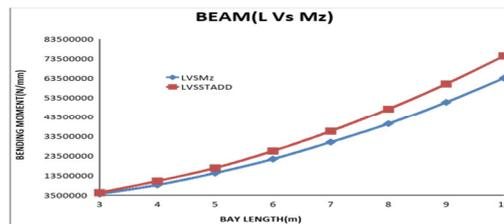
Figure 7 Bending moment in beam Vs Bay length
