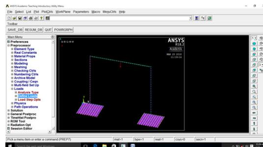
Figure 2 Building frame modeled in ANSYS
