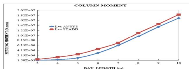
Figure 5 Bending moment in column Vs Bay length
