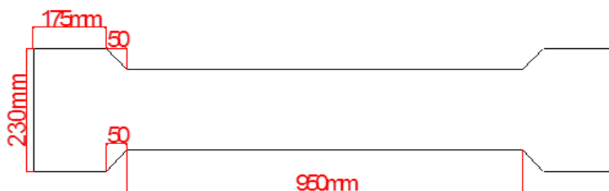
Figure 1 Schematic diagram of column cross-section with dimensions
