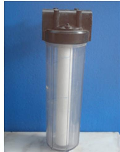
**Plate (1)** Multi Stage MBR with different porous Media, Radial flow system (e) poly propylene cartridge
