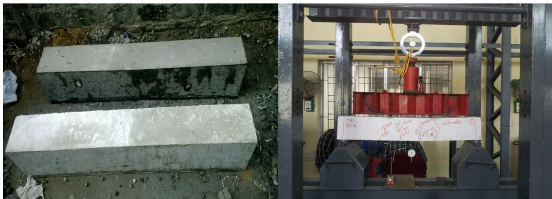
Figure 2 Testing of RC Beam
