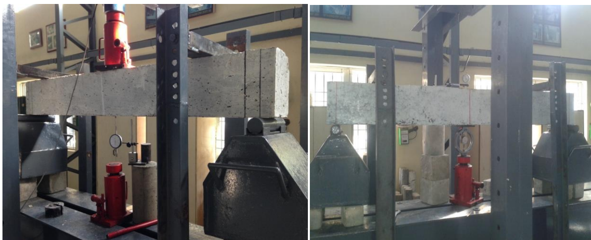
Figure 1 Test setup for cyclic loading
