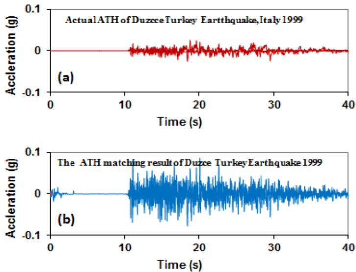
Figure 11 (a) The actual time history measurement result. (b) The matching time history which frequency characteristics agree with the attenuation law spectrum and different from frequency characteristics of actual time history.
