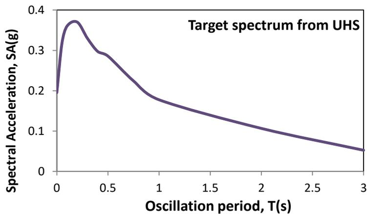
Figure 5 The uniform hazard spectrum of the point 110.4130<sup>0</sup>east; 7.6874<sup>0</sup>south.
