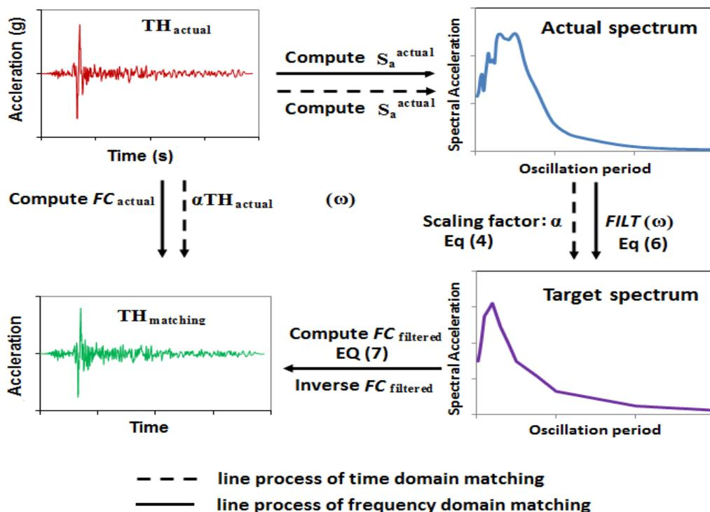
Figure 2 Methodology developed for spectral matching
