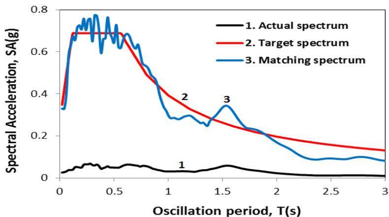
**Figure 14** Spectral matching with target spectrum is the UBC 1997 spectrum
