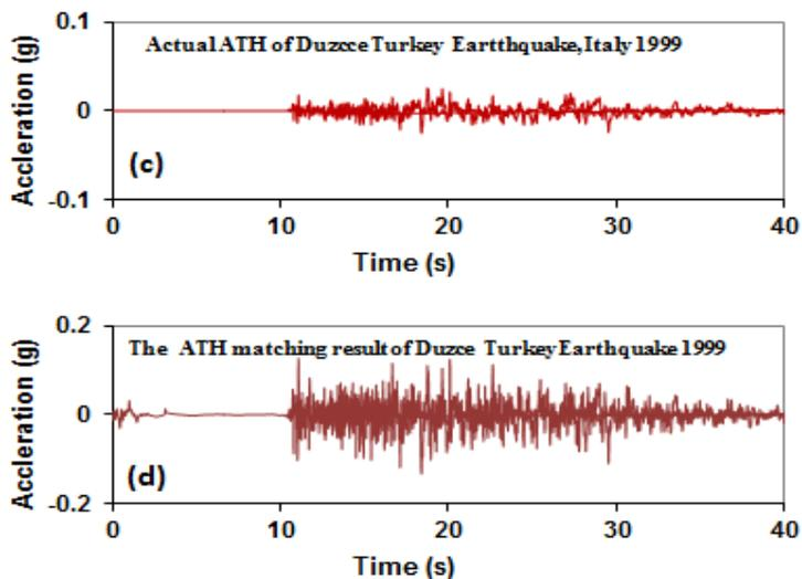
**Figure 13** (c) The actual time history measurement result. (d) The matching time history which frequency characteristics agree with the uniform hazard spectrum characteristics
