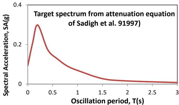
Figure 4 The attenuation response spectrum of Sadigh et al. (1997)
