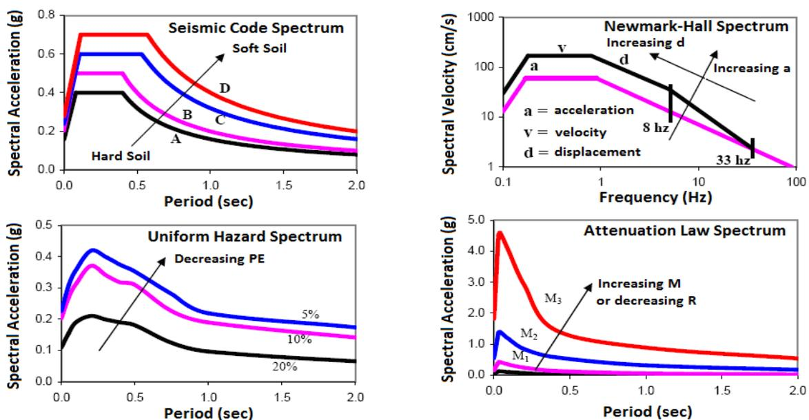
Figure 1 Response spectra for target spectrum
