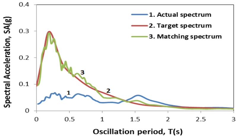
Figure 10 Spectral matching with target spectrum is the attenuation law spectrum
