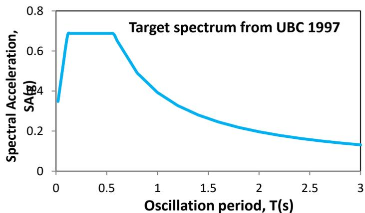
Figure 6 The UBC 1997 spectrum as target spectrum.
