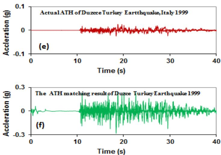
**Figure 15** (c) The actual time history measurement result. (d) The matching time history which frequency characteristics agree with the seismic code spectrum characteristics
