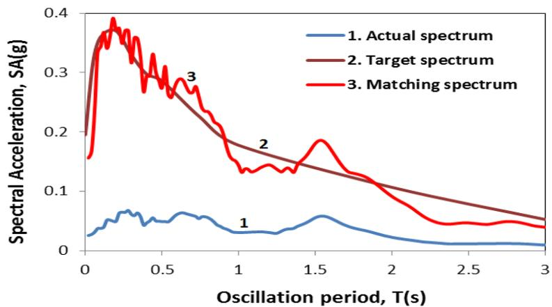
Figure 12 Spectral matching with target spectrum is the uniform hazard spectrum
