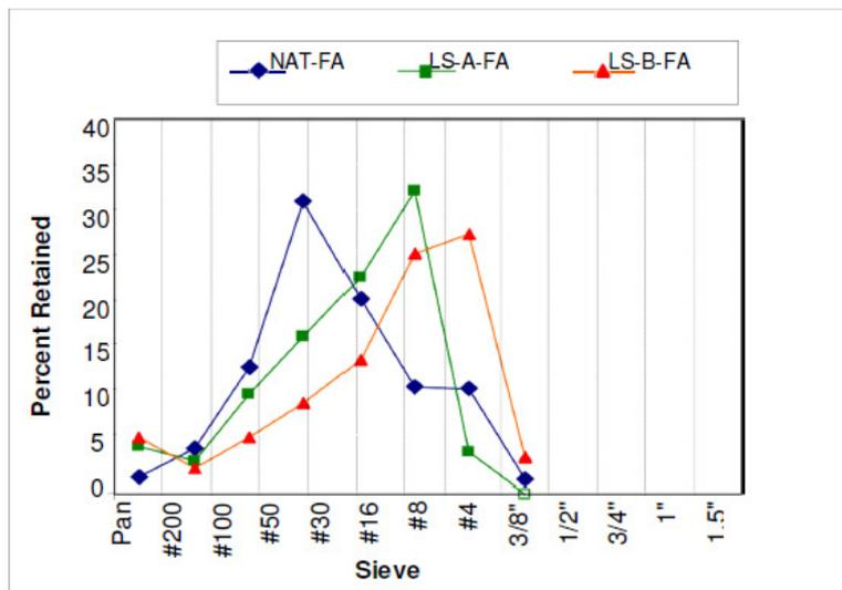
**Figure 4.2** Percent Retained for Fine Aggregate
