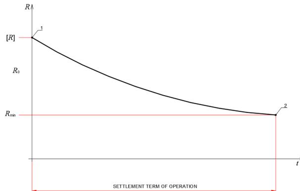
**Figure 1** Dependence "the bearing ability - time" for the designs operated in usual conditions
