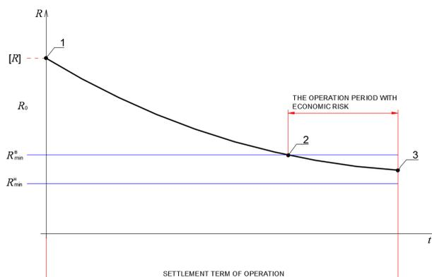
**Figure 2** Dependence "the bearing ability - time" for the designs operated in seismic conditions
