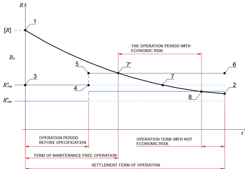
**Figure 5** Dependence "the bearing ability - time" for the designs operated in conditions increases of level of seismicity of the territory
