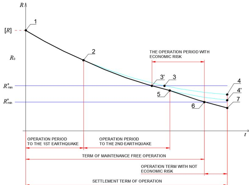
**Figure 3** Dependence "the bearing ability - time" in the conditions of seismic influences
