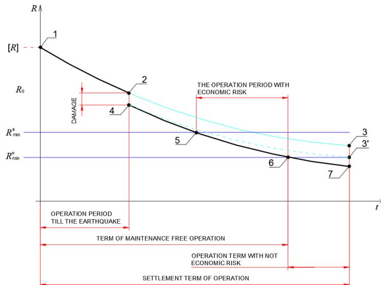
**Figure 4** Dependence "the bearing ability - time" at seismic influence of beyond design basis size
