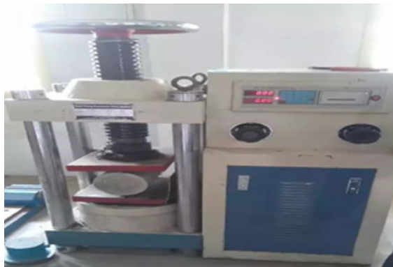
Figure 2 Split tensile testing of concrete cylinder
