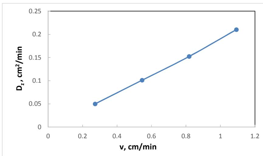
**Figure 2** The influence of interstitial velocity on the dispersion coefficient.
