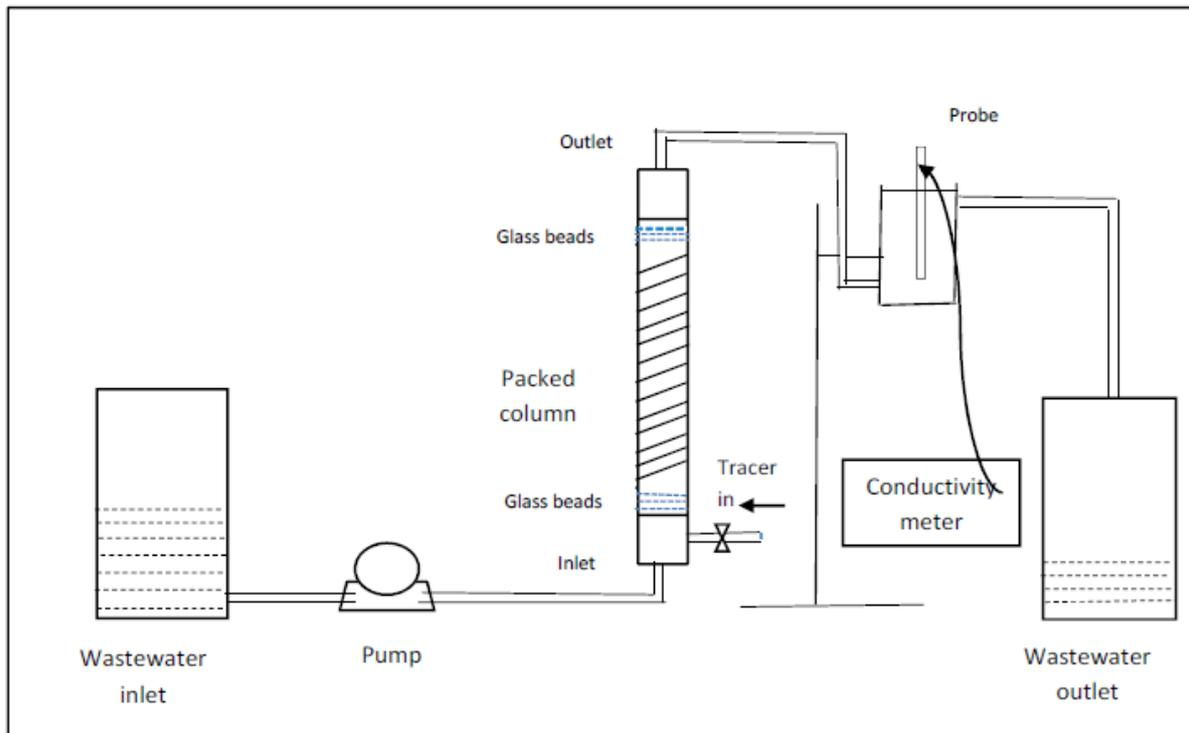
**Figure 1** The diagrammatic representation of RTD studies experimental arrangement
