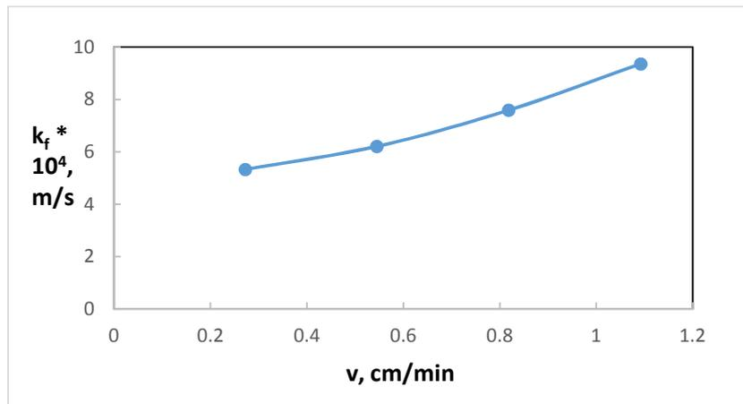
**Figure 3** The influence of interstitial velocity ( $v$ ) on the mass transfer coefficient ( $k_f$ ).
