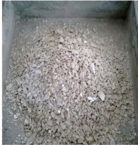
**Figure 2** Ceramic waste aggregate
