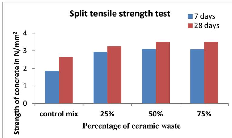
Figure 4 Split tensile strength test results
