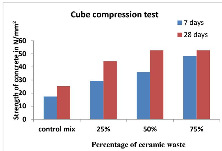
**Figure 3** Cube compressive strength test results
