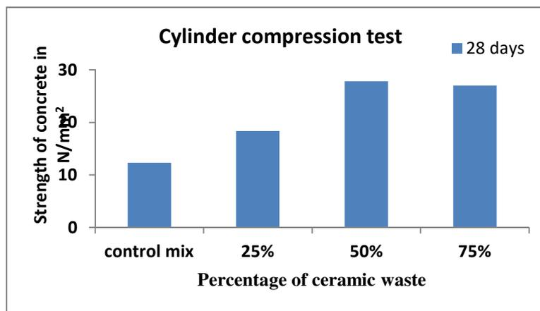
Figure 5 Cylinder compression test results
