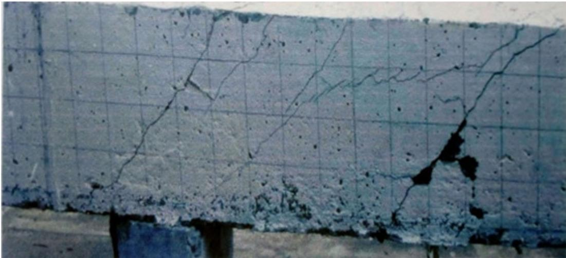
**Figure 7** Crack Pattern of beam with 1% steel fibres.
