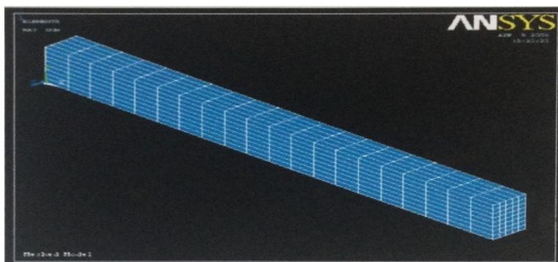
Figure 10 Meshed view of the beam
