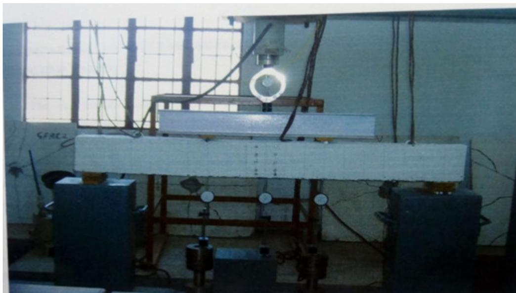
**Figure 6** Testing arrangement of beams
