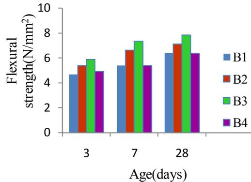
Figure 8 (b) Flexural strength of bacterial concrete with RHA and QD
