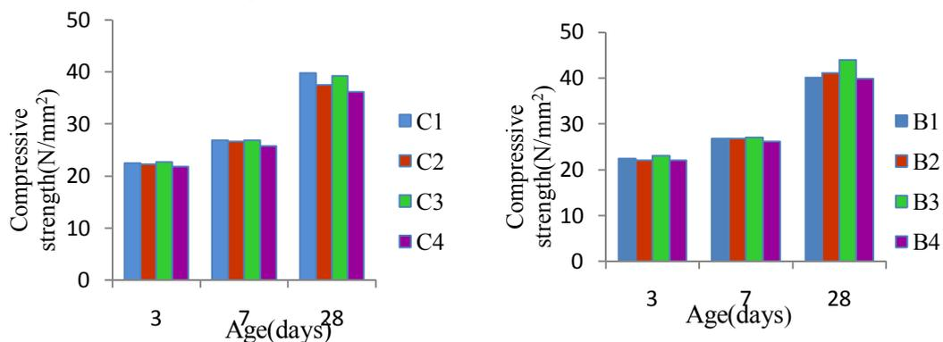
Figure 6 (a) Compressive strength of control concrete with RHA and QD Figure 6 (b) Compressive strength of bacterial concrete with RHA and QD
