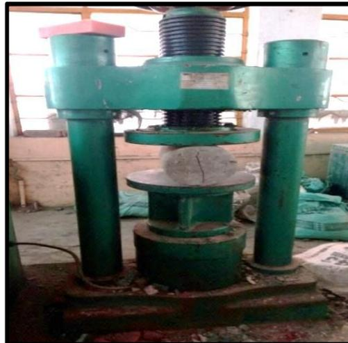
**Figure 4** Cylinder tested in compression testing machine
