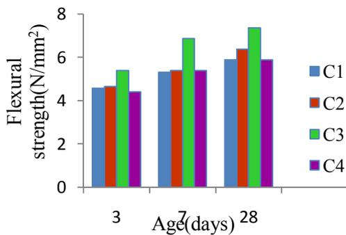
Figure 8 (a) Flexural strength of control concrete with RHA and QD
