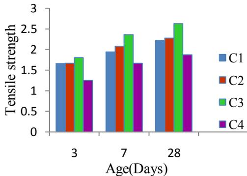
Figure 7 (a) Tensile strength of control concrete with RHA and QD
