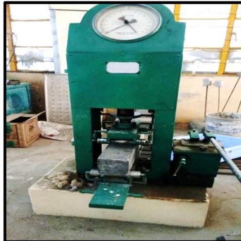
Figure 5 Prism tested in flexure testing machine
