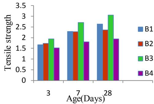
Figure 7 (b) Tensile strength of bacterial concrete with RHA and QD
