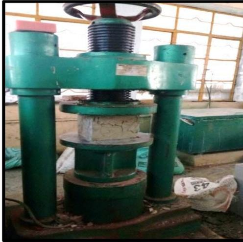
**Figure 3** Cube tested in compression testing machine
