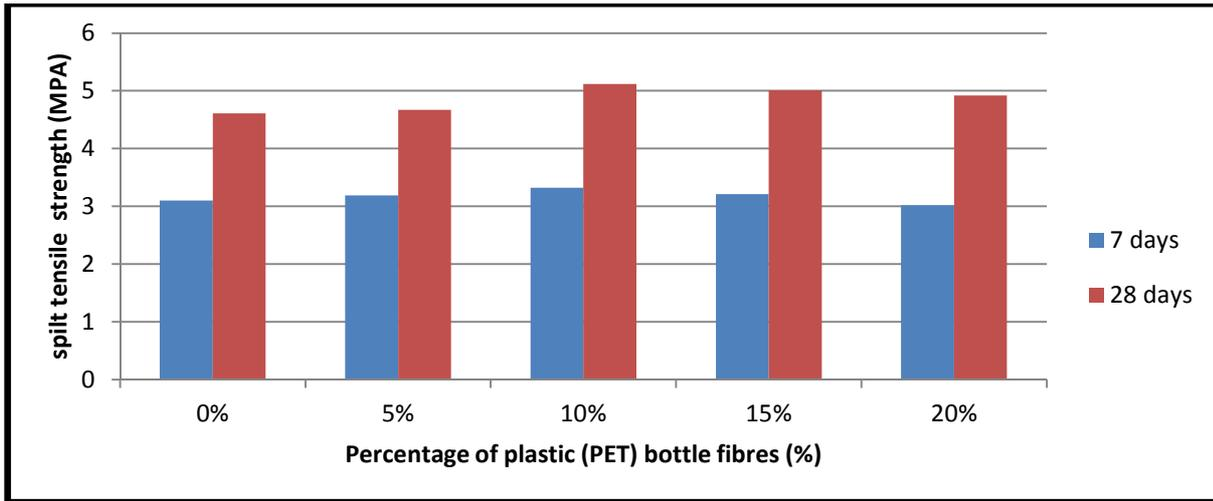
**Figure 11** Spilt tensile strength Vs Plastic fibres (%) for M30 grade of concrete
