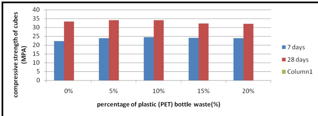
**Figure 6** Compressive strength Vs plastic waste for M25 grade of concrete
