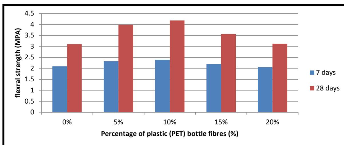
**Figure 8** Flexural strength Vs Plastic fibres (%) for M30 grade of concrete
