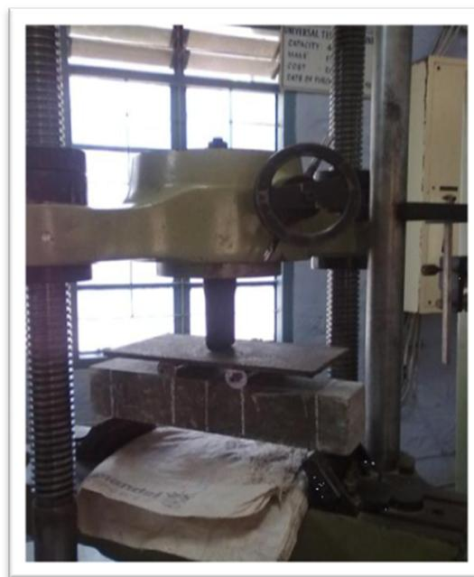
**Figure 3b** Flexural strength test set up
