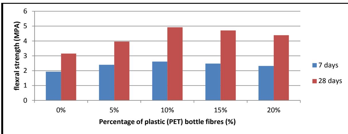
**Figure 10** Flexural strength Vs Plastic fibres (%) for M20 grade of concrete
