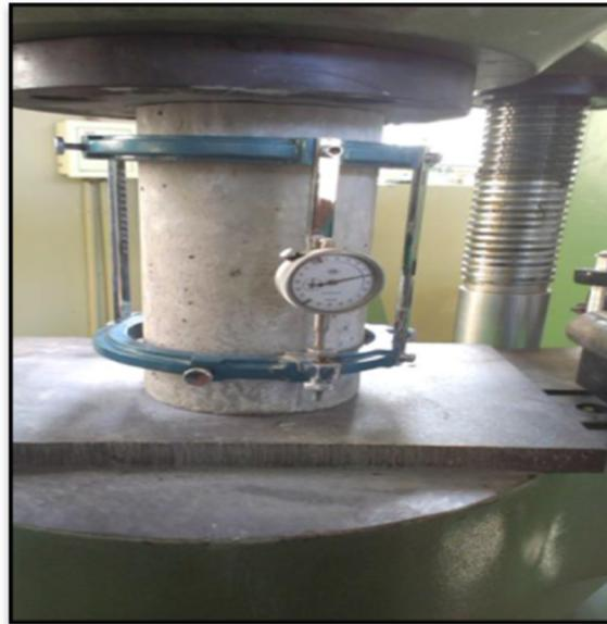
**Figure 3c** Split tensile strength test set up
