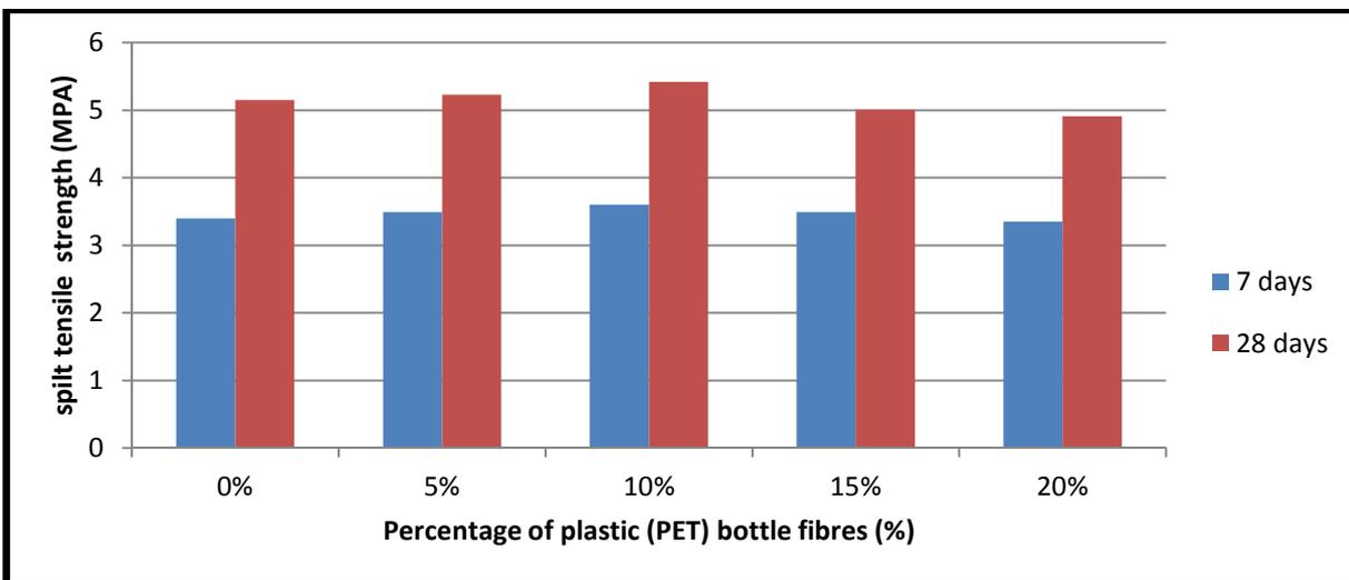
**Figure 12** Spilt tensile strength Vs Plastic fibres (%) for M25 grade of concrete
