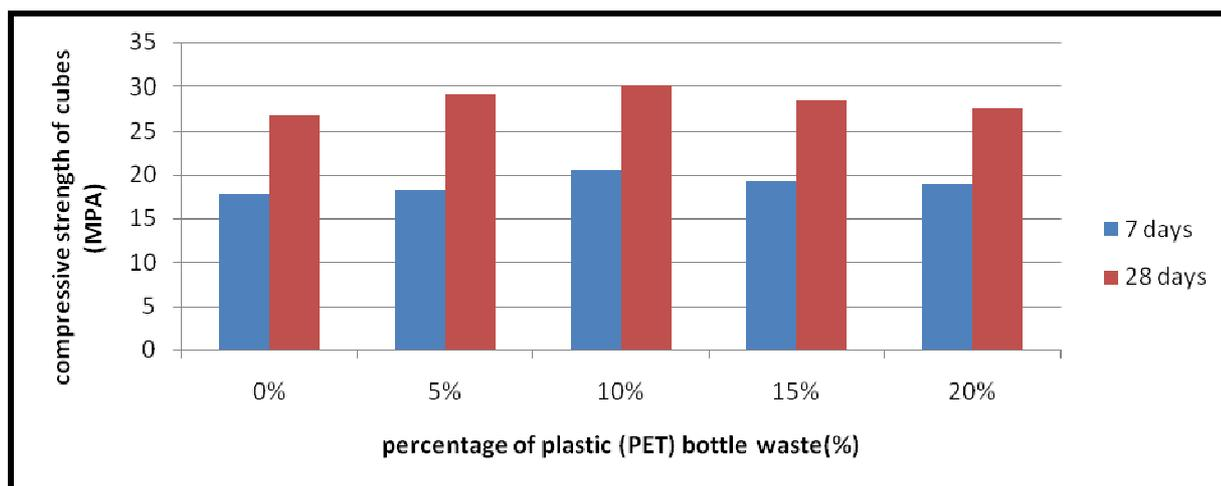
**Figure 7** Compressive strength Vs plastic waste for M20 grade of concrete
