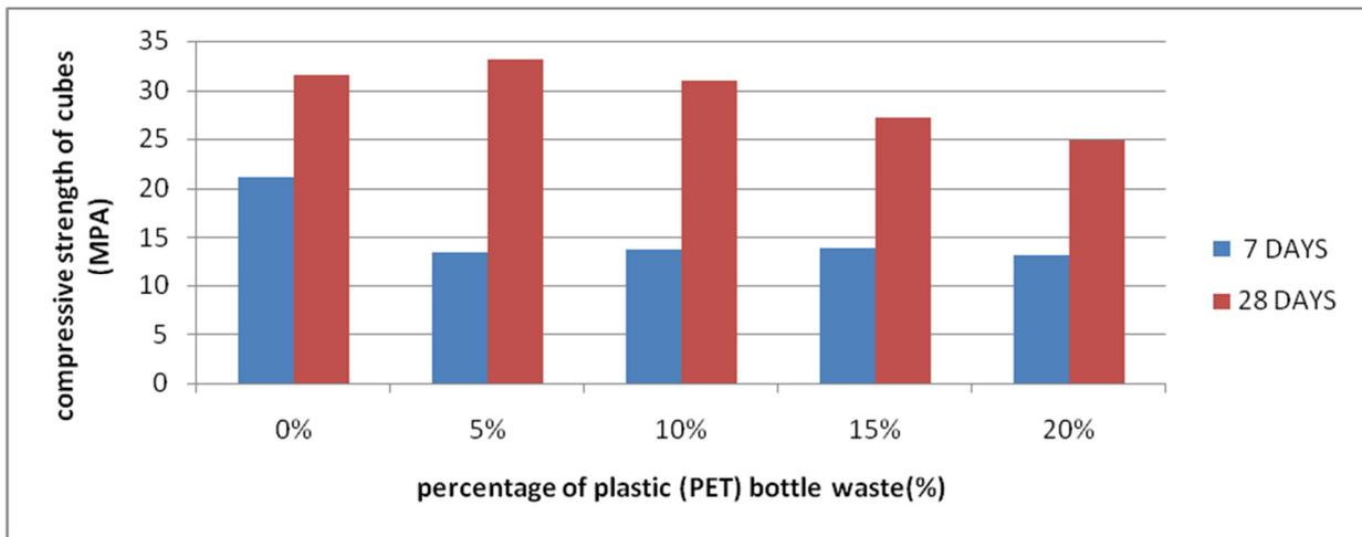
**Figure 5** Compressive strength Vs plastic waste for M30 grade of concrete
