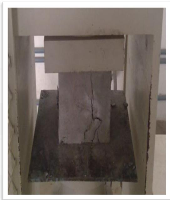
**Figure 3a** Compression test set up
