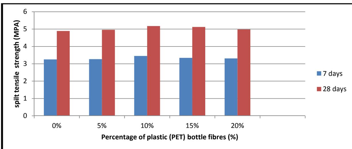
**Figure 13** Spilt tensile strength Vs Plastic fibers (%) for M20 grade of concrete
