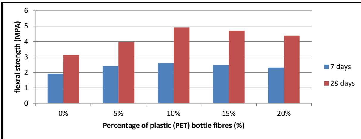
**Figure 9** Flexural strength Vs Plastic fibres (%) for M25 grade of concrete
