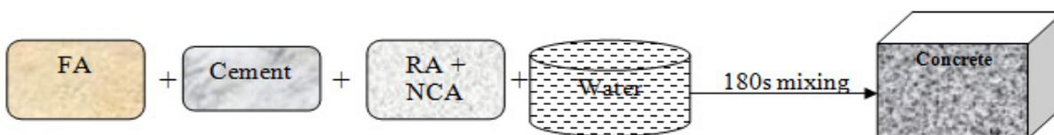
**Fig. 1 Normal Mixing Approach**
