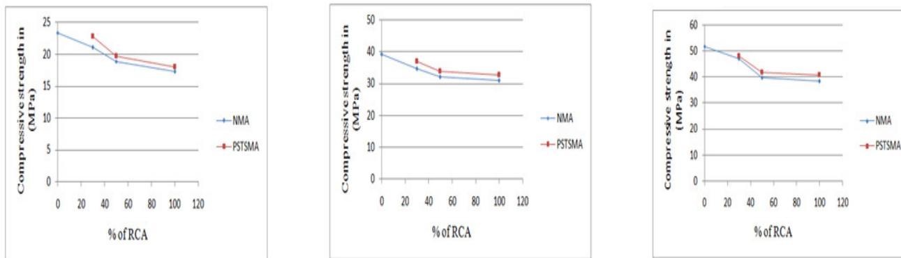
Comparison of compressive strength at 3 days age between NMA and PSTSMA Comparison of compressive strength at 7 days age between NMA and PSTSMA Comparison of compressive strength at 28 days age between NMA and PSTSMA
