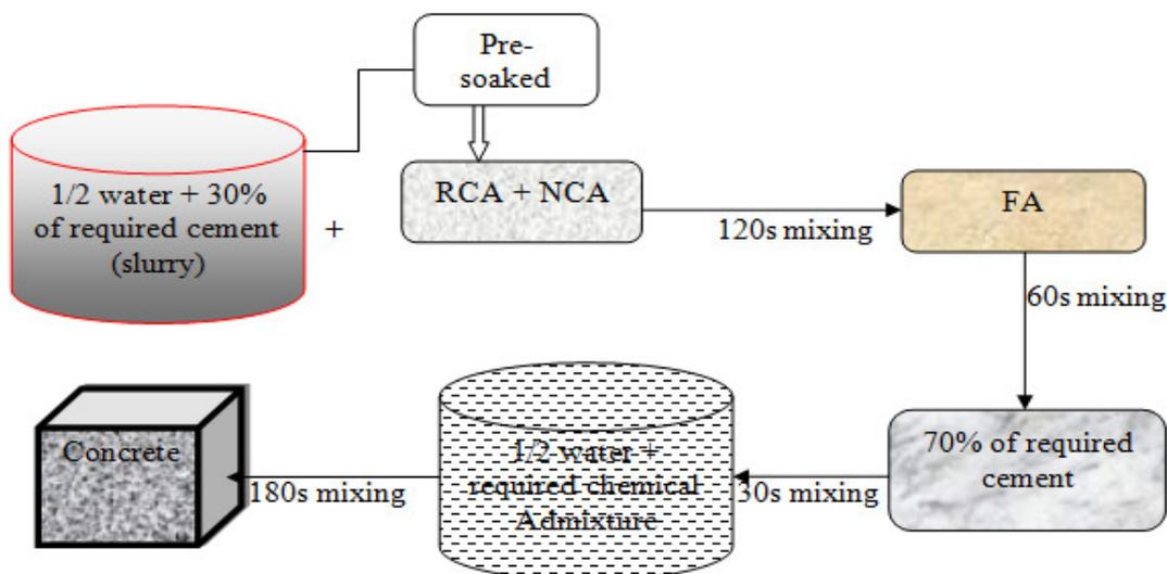
**Figure 2** Pre-soaked slurry two stage mixing approach.
