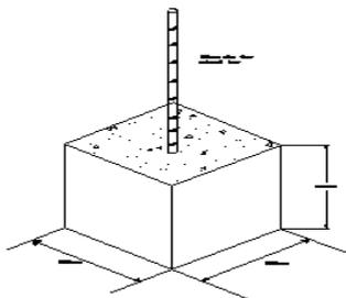
**Fig. 1:** Cube with 16mm diameter of tor steel rod embedded at center.
