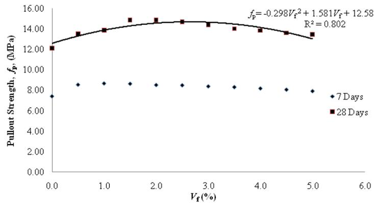
**Fig. 2: Variation of Pullout Strength With Respect to Fiber Content**
