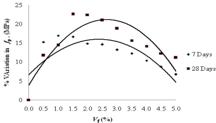
**Fig.3: Percentage Variation in Pullout Strength on Prisms Over Controlled Concrete With Respect to Fiber Content ( $V_f$  %)**
