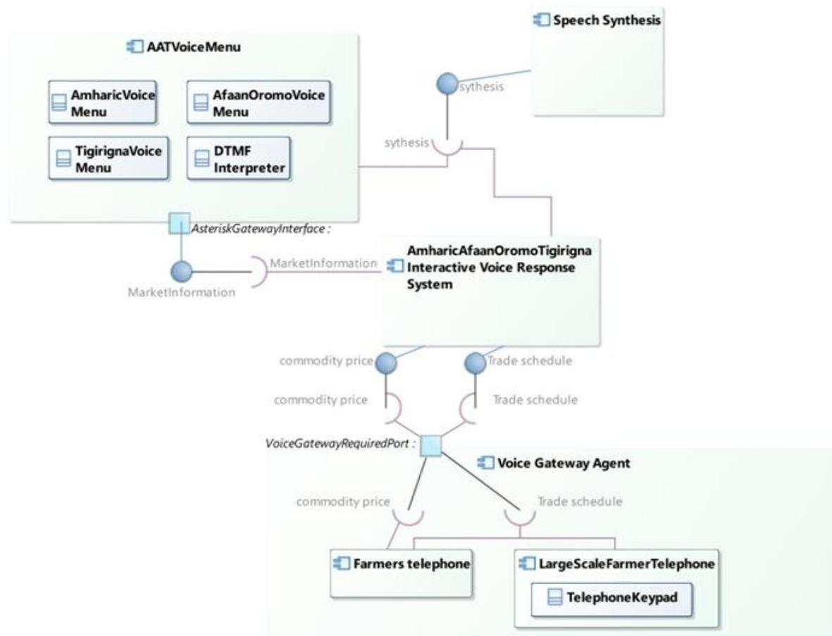
Figure 2 Layered representation on proposed model
