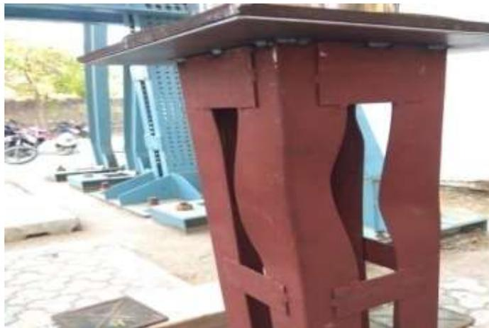
**Figure 5** Buckling mode
