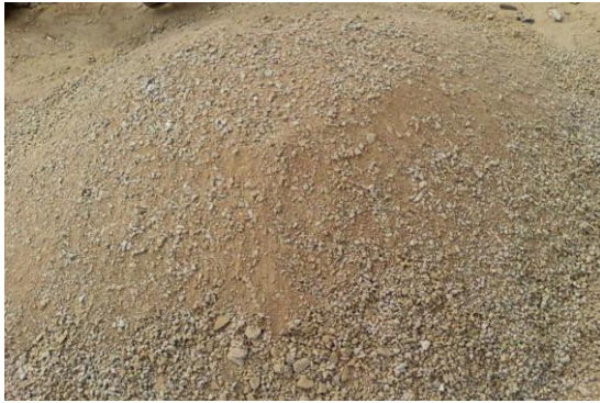
Figure 2 Stockpiling of Demolished CD
