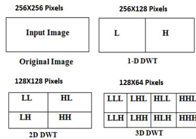
Figure 10 Image decomposition in 1D, 2D and 3D-DWT
