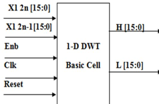
Figure 4 Pin Layout of 1D DWT
