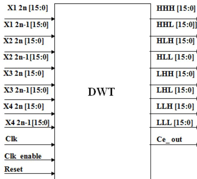
**Figure 3** Pin Layout of Proposed Architecture
