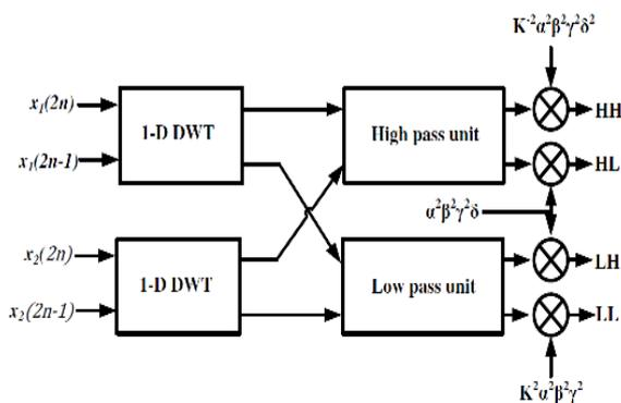
Figure 8 Structure of 2D DWT
