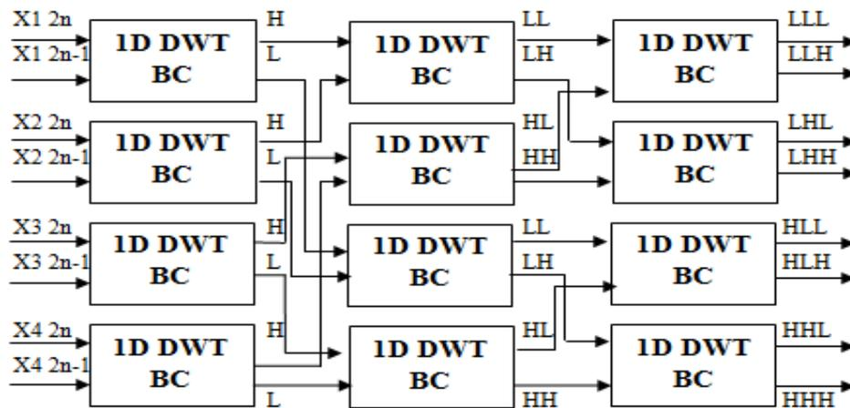
**Figure 9** Proposed 3D-DWT VLSI Architecture
