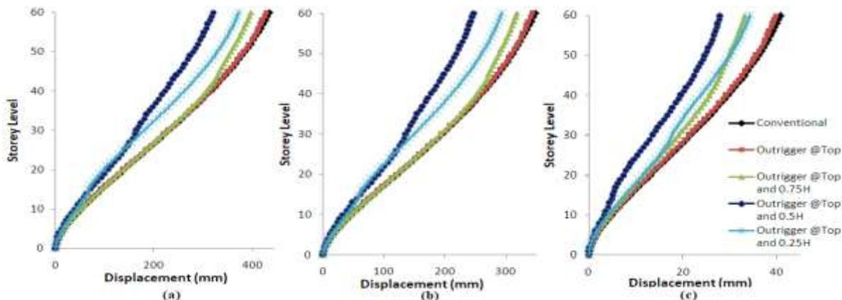
Figure 6 Lateral Displacement for 60 storey models by (a) ESM (b) RSM (c) THA
