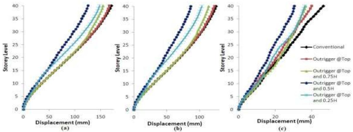
**Figure 5** Lateral Displacement for 40 storey models by (a) ESM (b) RSM (c) THA
