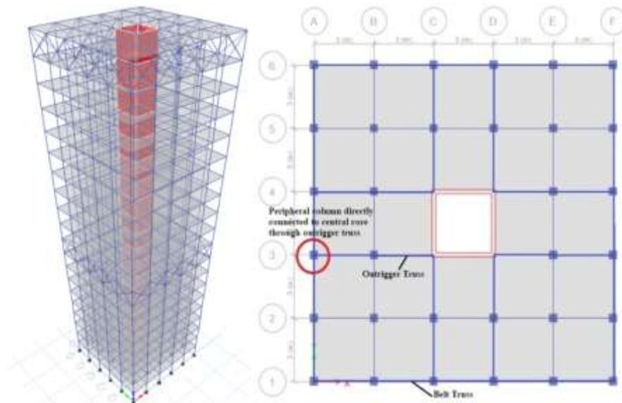
**Figure 2** 3D model and plan of the 20 storey building in ETABS software
