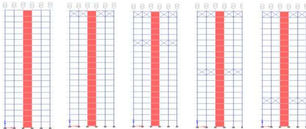
**Figure 3** Elevation of the different 20 storey structural configurations
