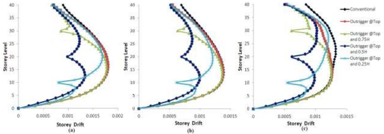
Figure 8 Storey drift for 40 storey models by (a) ESM (b) RSM (c) THA
