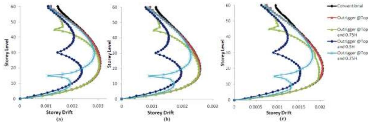
Figure 9 Storey drift for 60 storey models by (a) ESM (b) RSM (c) THA
