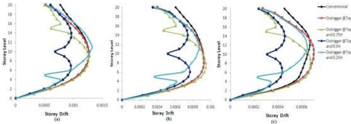
Figure 7 Storey drift for 20 storey models by (a) ESM (b) RSM (c) THA
