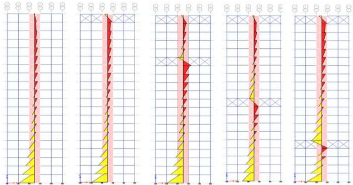
**Figure 10** Variation of moment in the central core along the height for different structural configurations of 20 storey by Equivalent Static Method
