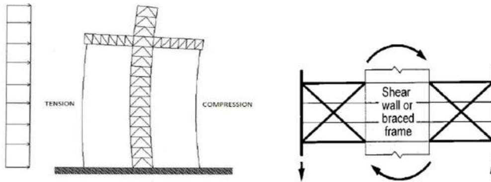
**Figure 1** Mechanism of outrigger system
