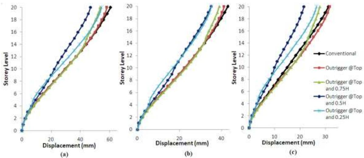
**Figure 4** Lateral Displacement for 20 storey models by (a) ESM (b) RSM (c) THA
