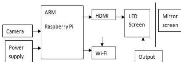
**Figure 2** Block diagram of Proposed System
