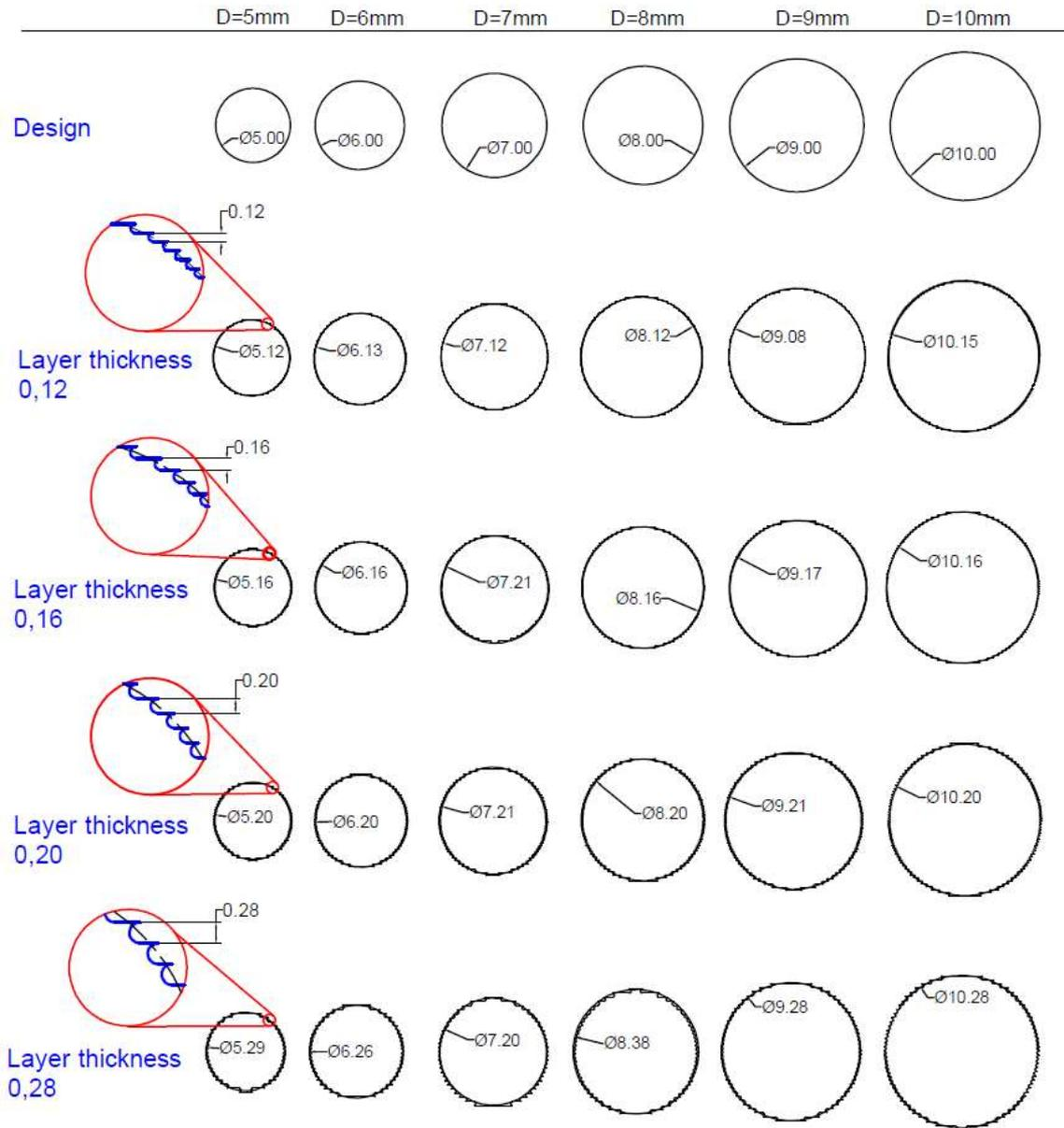
**Figure 6** Simulation of curve profile in design and 04 printing modes.
