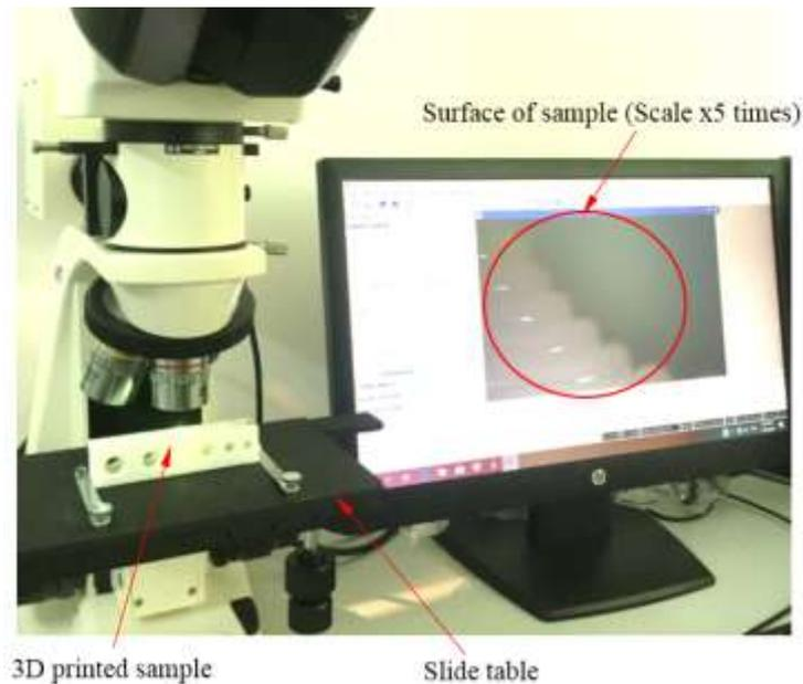
**Figure 3** Measurement setting of the sample on microscope optical machine
