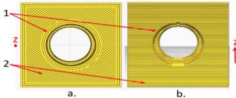
**Figure 1** Simulation of the layers in printing by Ultimaker Cura.
