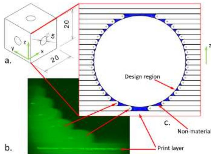
**Figure 5** Model of vertical section of sample with printed layers; a. part design; b. printed sample; c. model develop
