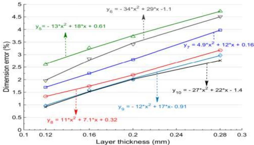
**Figure 7** Simulate size errors under different print conditions
