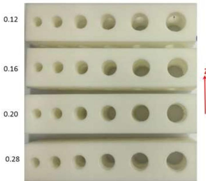
**Figure 2** Samples was printed from 3D printer under different conditions.
