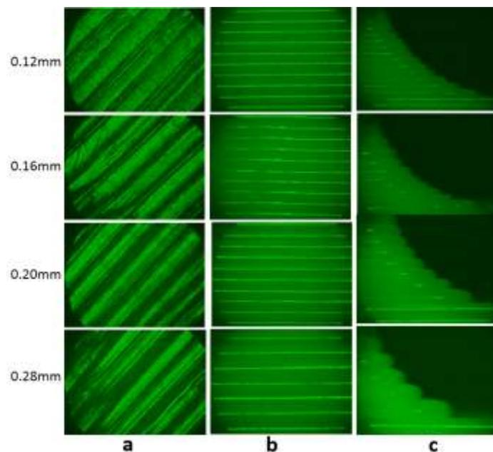
**Figure 4** Image of sample surface were printed under different layer thickness;
