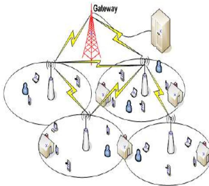
**Figure 1** Architecture of the Wireless Mesh Network
