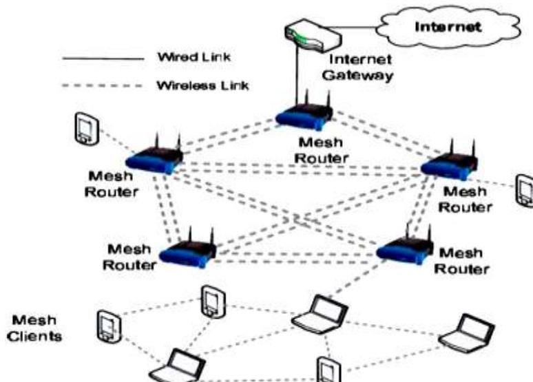
Figure 4 Hybrid Mesh Architecture
