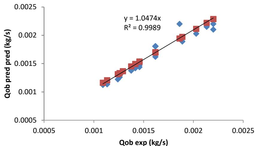
**Figure 6** Comparison of predictive material output capacity ( $Q_{ob}$  pred) with experiments ( $Q_{ob}$  exp) of ANN Testing
