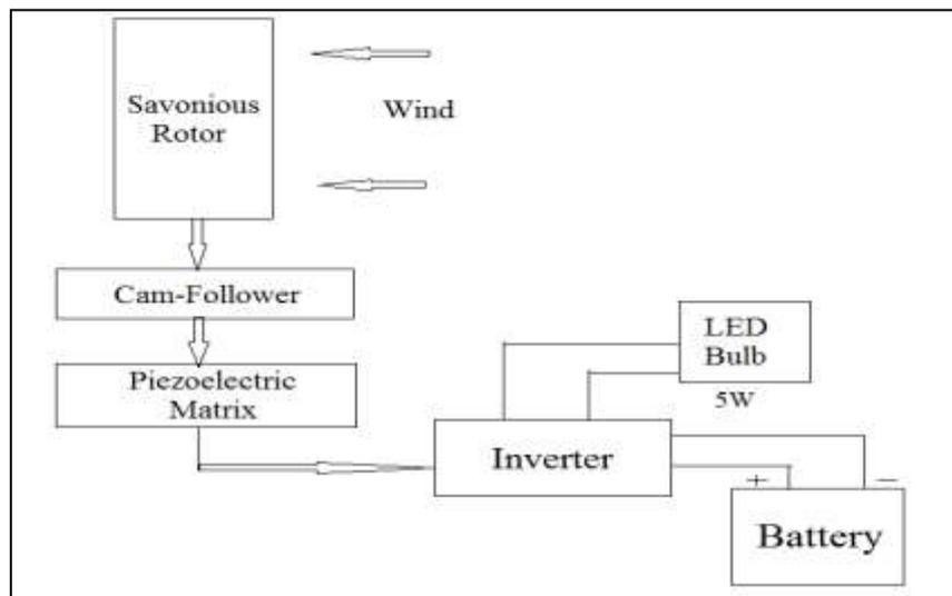
**Figure 1** Experimental set up using Piezoelectric Module
