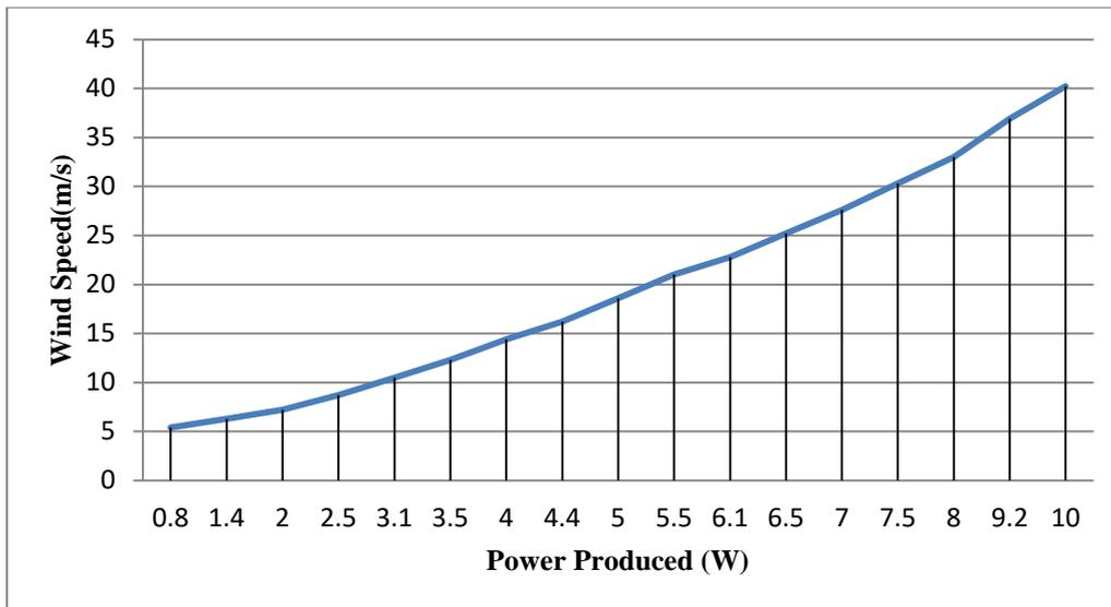
**Graph 2** Wind Speed vs Power produced
