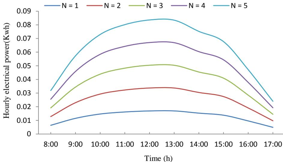
**Figure 4** Change in per hour electrical power outcome at flow of fluid mass / unit time 40 g/s and water depth = 14 cm for a standard day of July month
