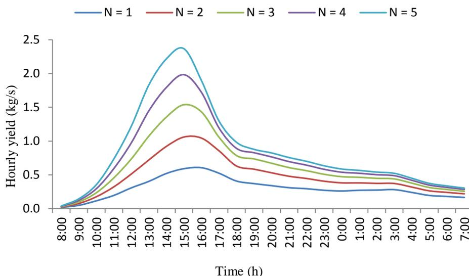
**Figure 2** Distribution of per hour yield with flow of fluid mass per unit time at flow of fluid mass = 40 g/s and water depth = 14 cm for a standard day of July
