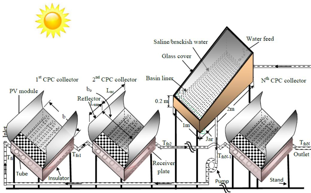
**Figure 1** Depiction of SSS desalting plant incorporated via N partially covered PVTCPs
