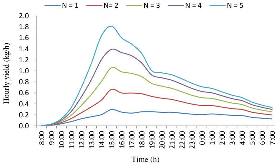
**Figure 3** Change in per hour production with flow of fluid mass per unit time at flow of fluid mass = 40 g/s and water depth = 14cm for a standard day of December month
