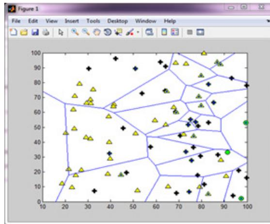
**Figure 8** Network topology after iteration and cluster formulation (maximum number of dead nodes detected)
