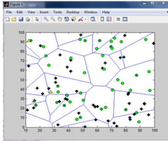
**Figure 7** Network topology with minimum number of dead nodes detected
