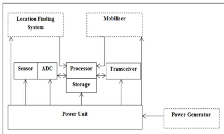
**Figure 1** Components of a sensor node
