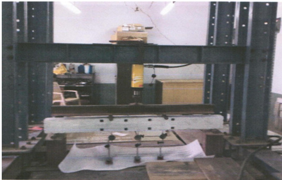
Figure 1 Loading Frame and test set up
