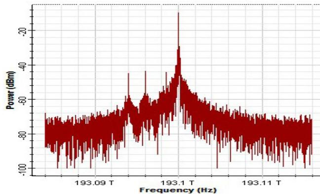
**Figure 5** Spectrum of OSSB modulated signal
