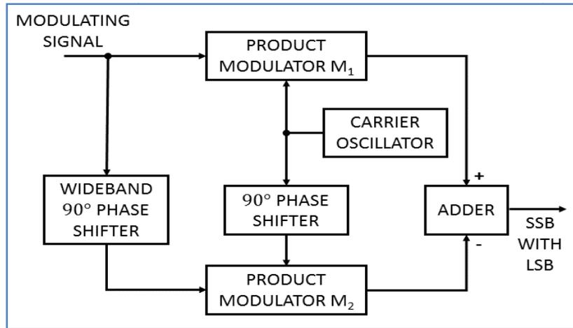
**Figure 2** Basic Structure of SSB generation
