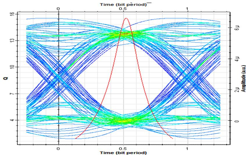
**Figure 7** Eye pattern of the received signal
