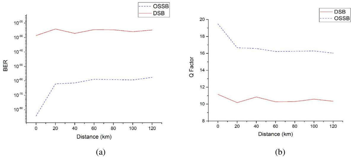
**Figure 6** Comparison of BER for DSB and OSSB system (a) BER and (b) QFactor.
