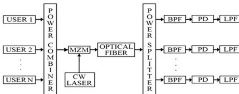
**Figure 1** Block Diagram of SCM
