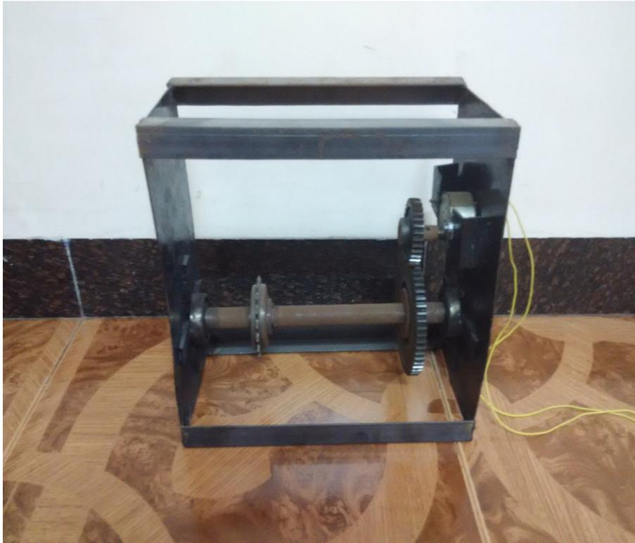
**Figure 1** Actual model with gears, sprocket and motor
