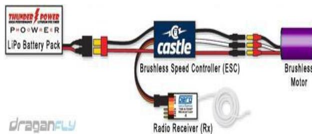
**Figure 2** Connection of Brushless Motor, ESC & LiPo Battery
