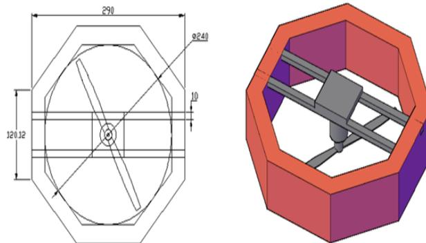
**Part 3 Back Motor Mount Design [PROPULSION OR THRUST] OF RC-ACV [G-1] 2015**
