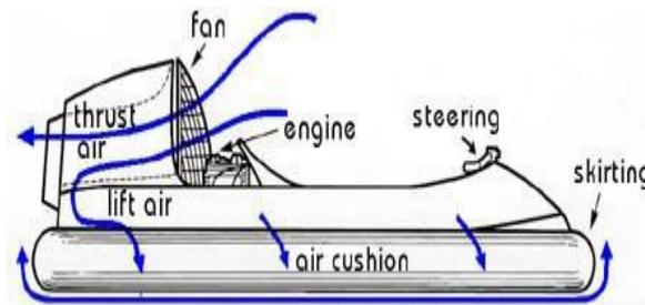
**Figure 1** Sketch of Working Principle of Hovercraft
